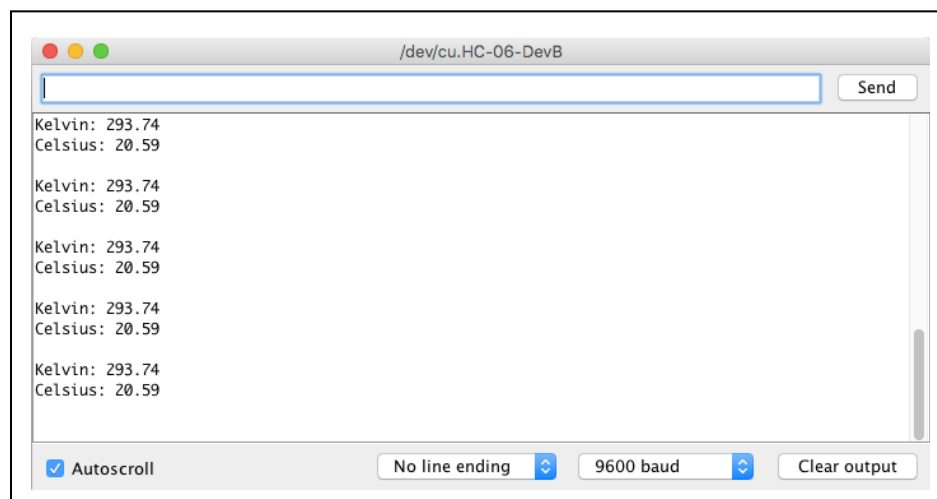
Figure 6 – Temperature data received via Bluetooth on computer console
