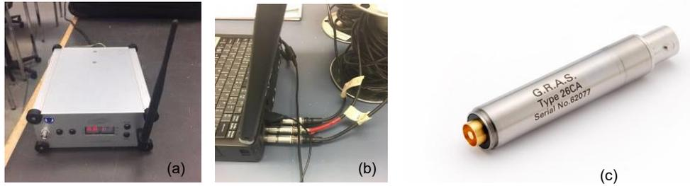
Figure 94: (a) Sound generator/sound amplifier, (b) A Soundbook with 3 channel outputs, (c) 1/2" microphones (G.R.A.S. 26CA).
