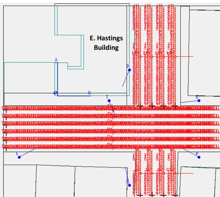
Figure 57: Omni array source set-up of E. Hastings configuration in the ODEON model.
