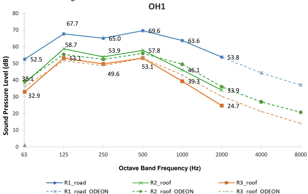
Figure 71: The OH1 design tool configuration spectrum analysis
