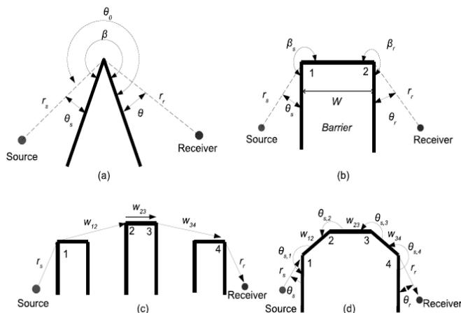
Figure 5: Four different building configurations that simplified a different diffraction function from source to receiver: (a) single, (b) double, (c) and (d) multiple. (Wei et al., 2015)
