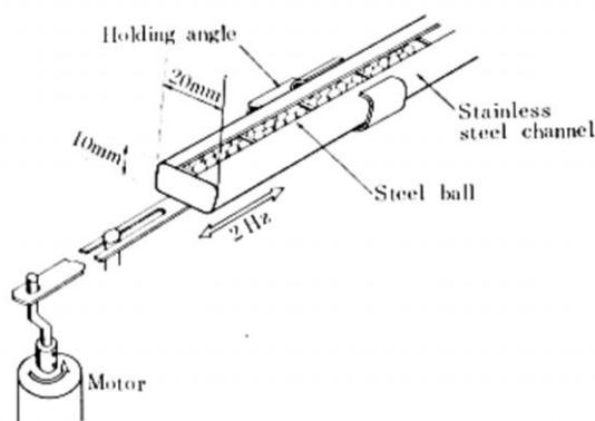
Figure 20: Details of line source set-up.
