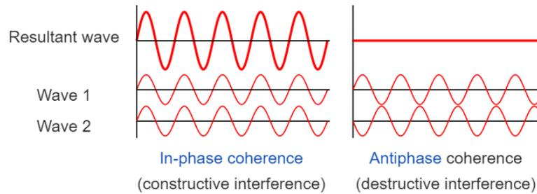
**Constructive interference** occurs when the phase difference between the waves is a multiple of  $2\pi$ .
