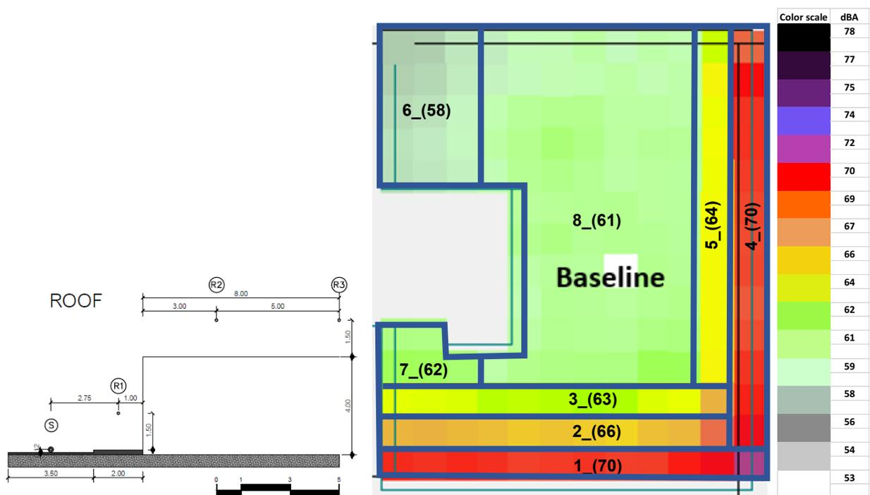
Figure 83: Sonic Subzone of Baseline ROOF configuration.
