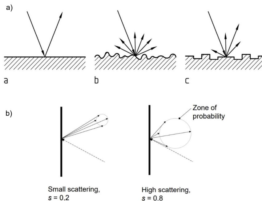
Figure 8: (a) Specular and diffuse reflection, (b) Scattering as weight vectors of surface reflection and the size of vectors. (Keränen et al., 2003)
