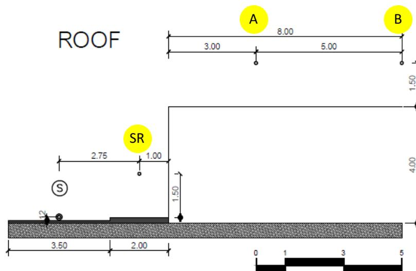
Figure 49: A baseline street-to-roof configuration.
