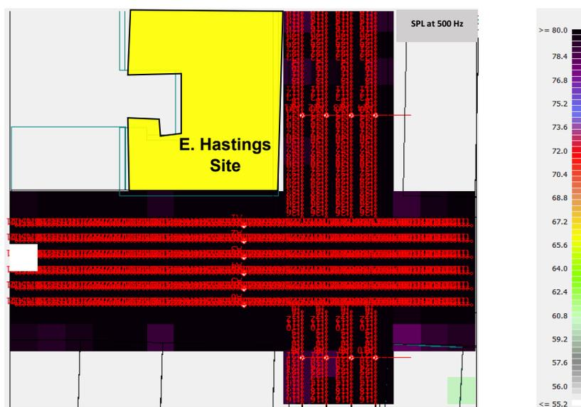
Figure 76: Colored grid response to SPL at 500 Hz resulting after the line source arrays had been assigned in ODEON.
