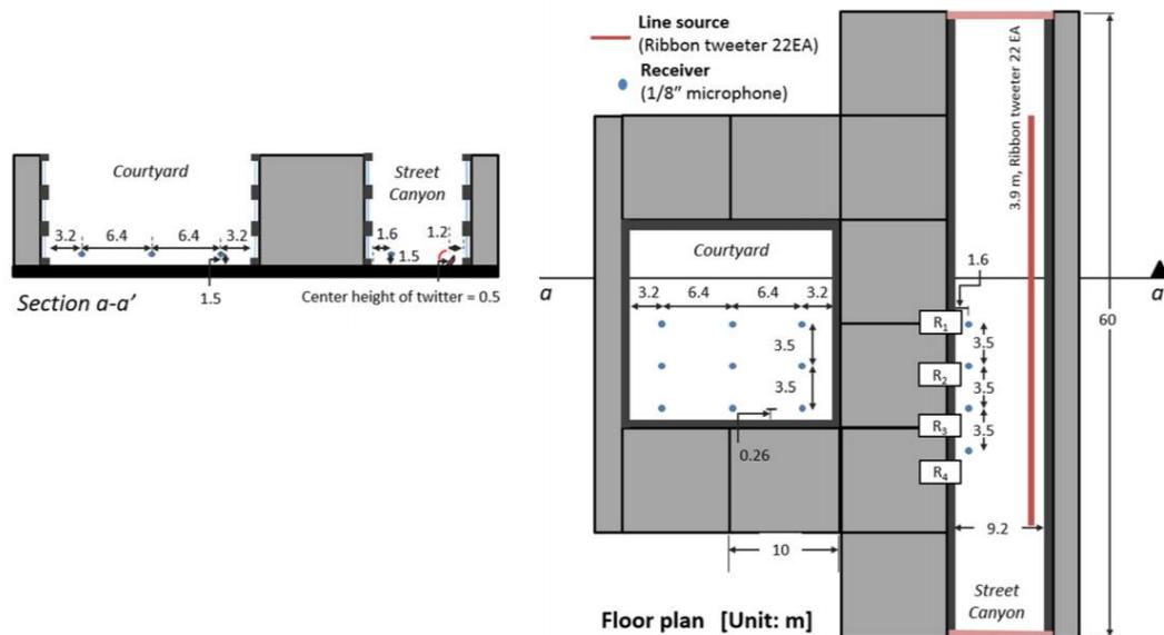
Figure 25: Reference configurations of an urban scale model, sources, and receiver positions. (Jang et al., 2015)
