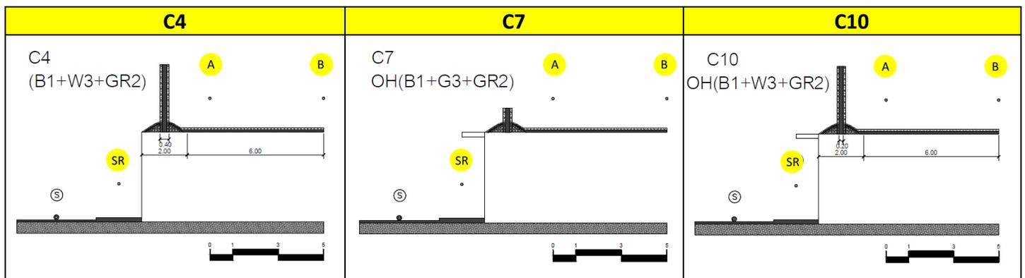
Figure 88: Complex configurations that showed the highest increased attenuation at Receiver B in the design tools investigation.
