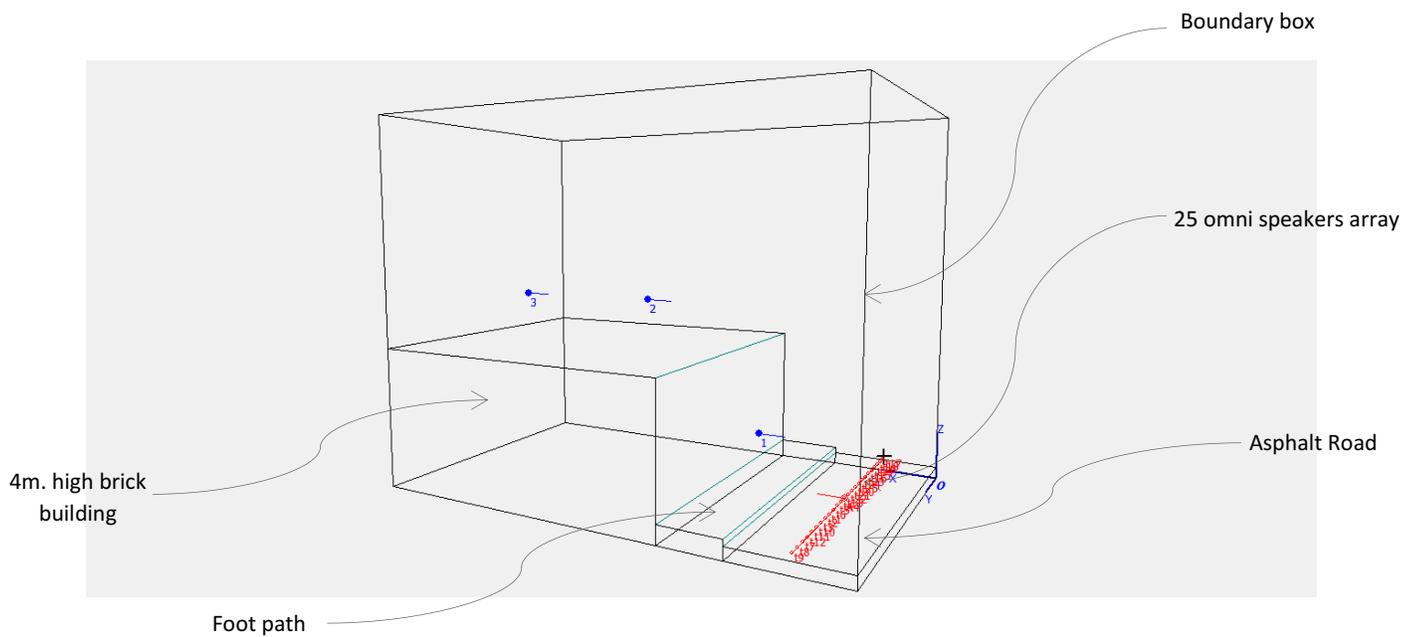
Figure 46: The perspective of the 25 omni-directional speakers array set-up of the baseline ROOF configuration model in ODEON.
