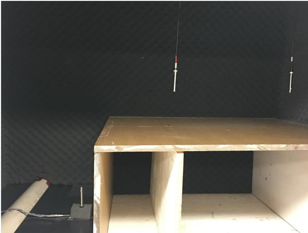
Figure 43: The picture illustrates a 1:10 scale model street-to-roof configuration (Baseline ROOF) and source receiver positions.
