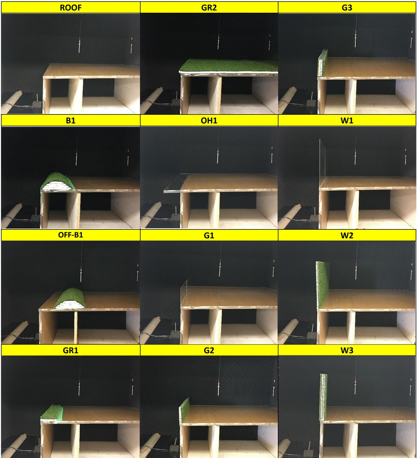
Figure 53: ROOF and single-design tool configurations for the 1:10 scale model tested in the anechoic chamber.
