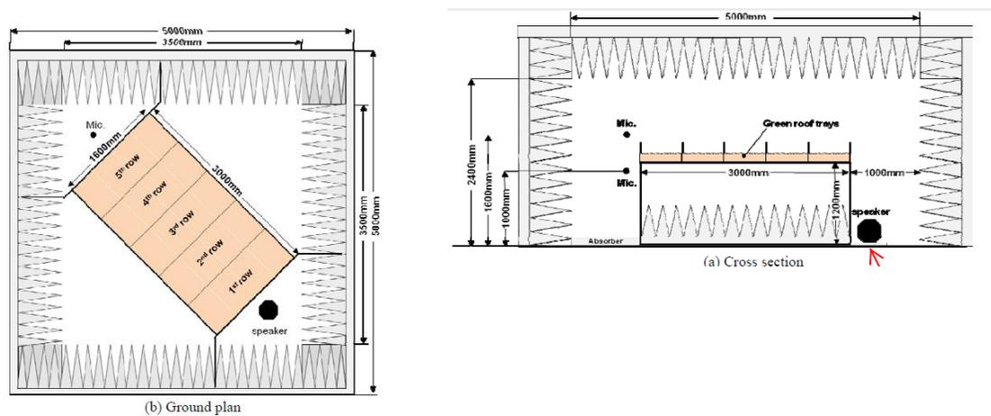
Figure 24: The cross-section and plan view of the scale model test in an anechoic chamber. (Yang et al., 2010)
