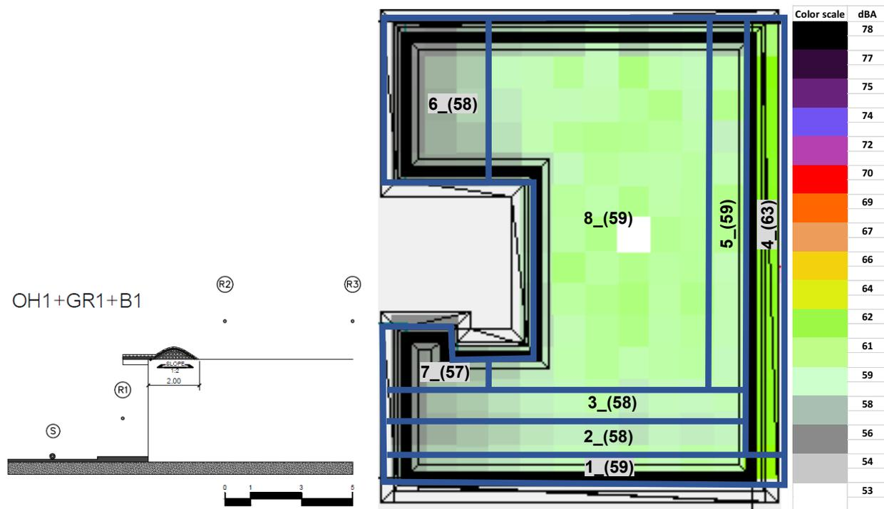
Figure 86: Sonic Subzone of OH1 +GR1+B1 configuration,
