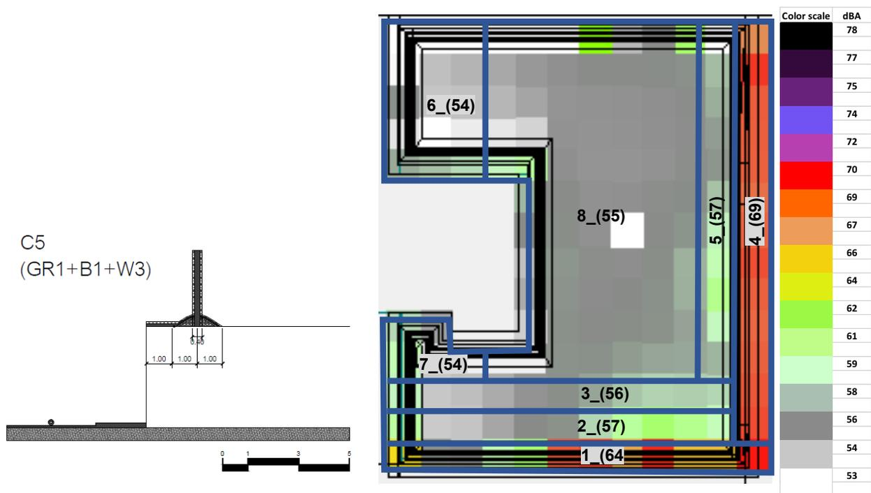
Figure 87: Sonic Subzone of C5, GR1+B1+W3 configuration,
