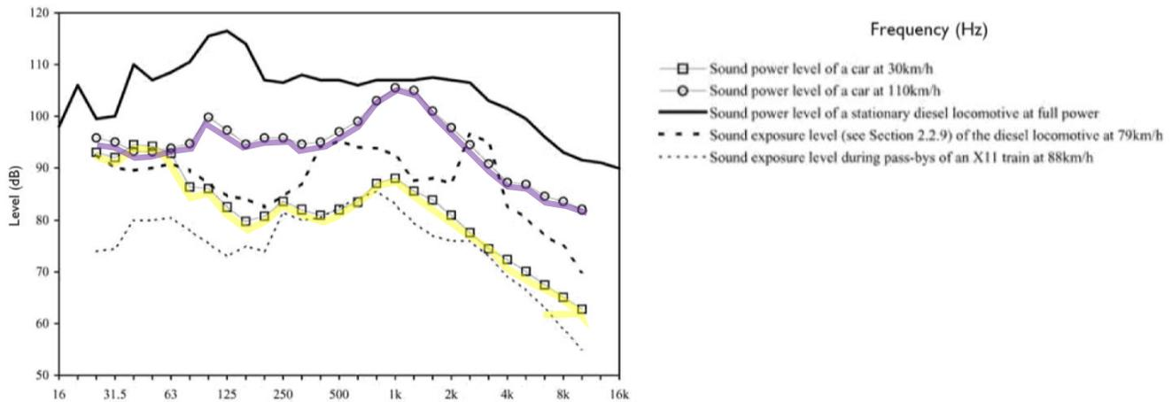
Figure 2: Typical spectra of car and train noise. (Kang, J., 2006)
