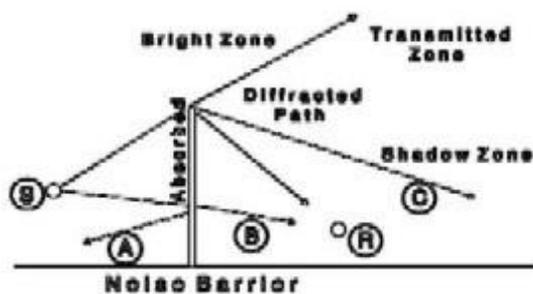
Figure 17: Various components of noise
