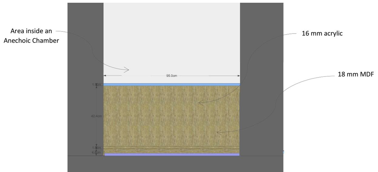
Figure 45: Construction of a 1:10 scale model street-to-roof configuration and Source receiver positions (side elevation).
