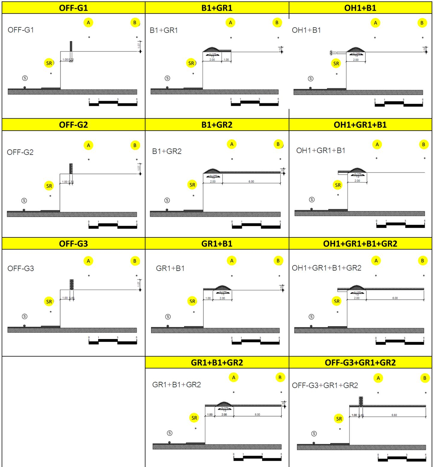
Figure 51: Off-set guard configurations, double- and triple-design tool configurations.
