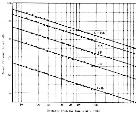
Figure 22: SPL as a function distance from the source.
