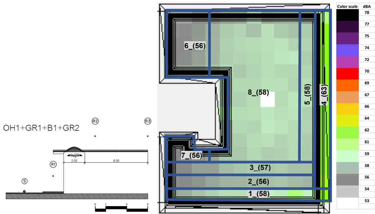
Figure 85: Sonic Subzone of OH1+GR1+B1+GR2 configuration,
