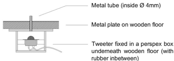
Figure 23: Point source detail set-up. (Dragonetti et al., 2011)
