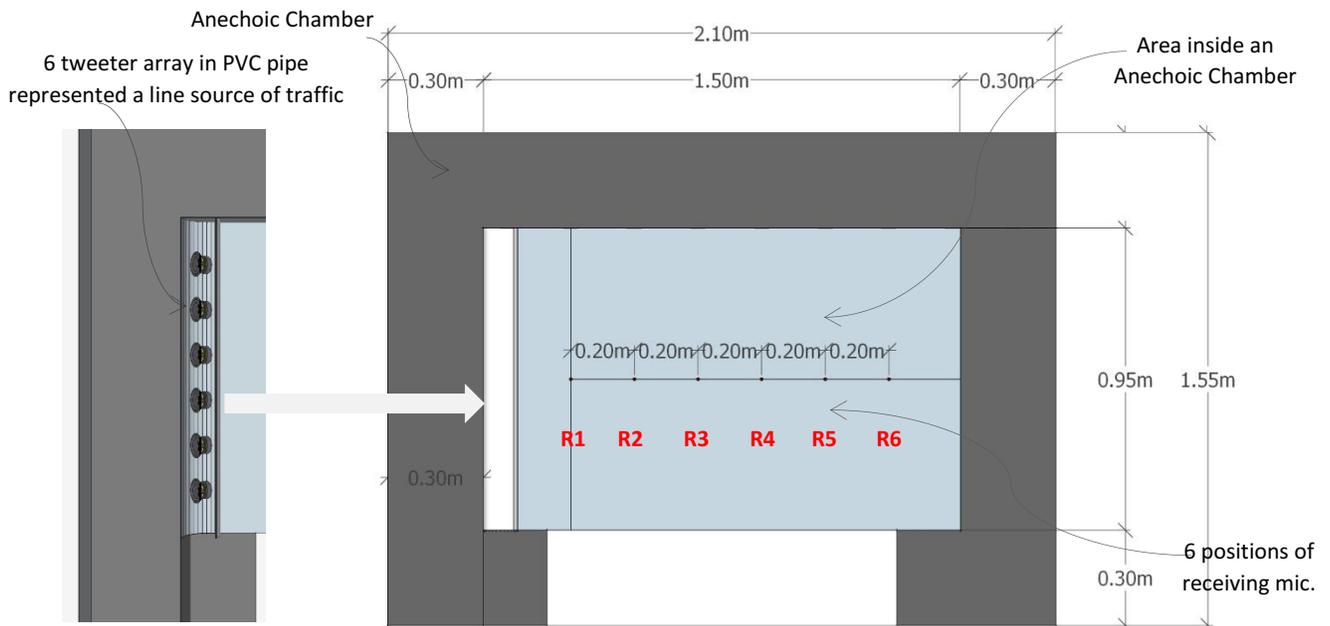
Figure 39: Top view of source modelling experiment set-up in the anechoic chamber.
