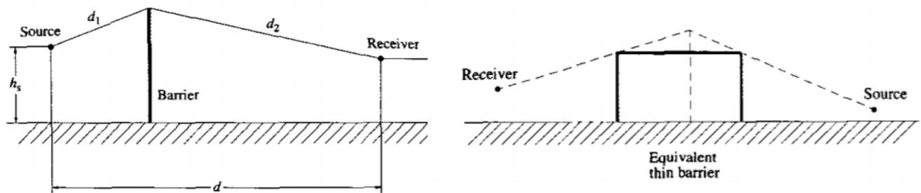
Figure 15: Geometry of sound propagation over a barrier. A thick barrier is equivalent to thin barrier. (Lines and Peng, 1995)
