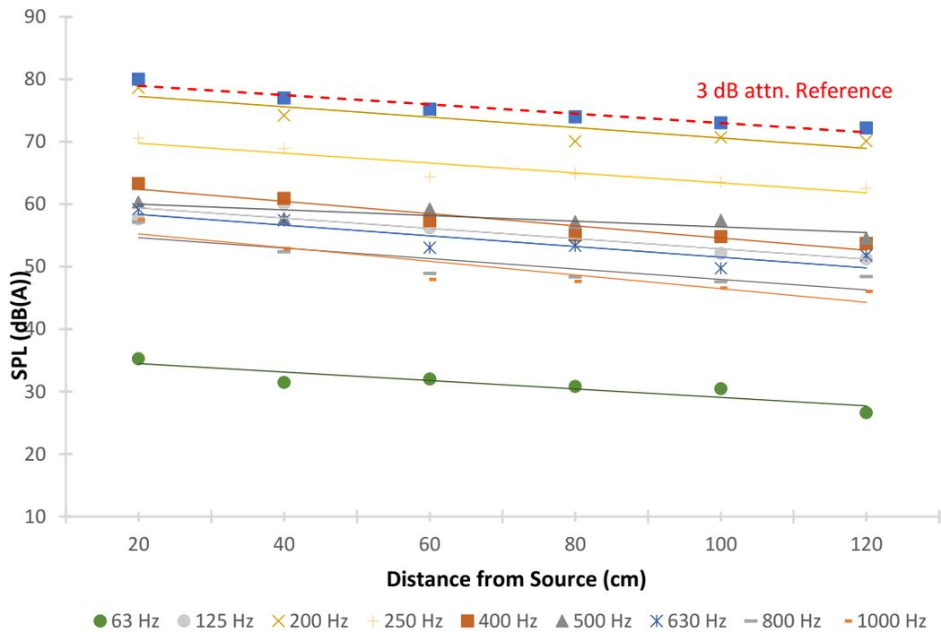
Figure 61: SPL as a function of distance from the source in the frequency range that shows 3 dB attn. per doubling the distance.
