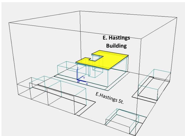
Figure 56: Perspective view of E. Hastings building configuration model in ODEON.
