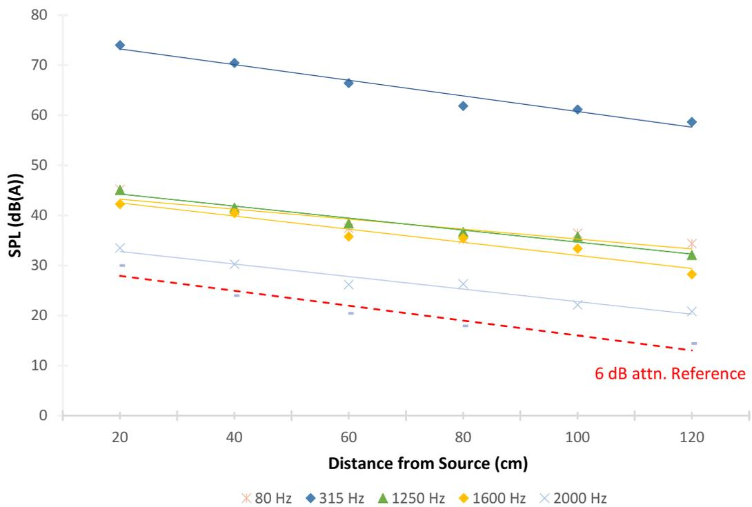
Figure 62: SPL as a function of distance from the source in the frequency range that shows 6 dB attn. per doubling the distance.
