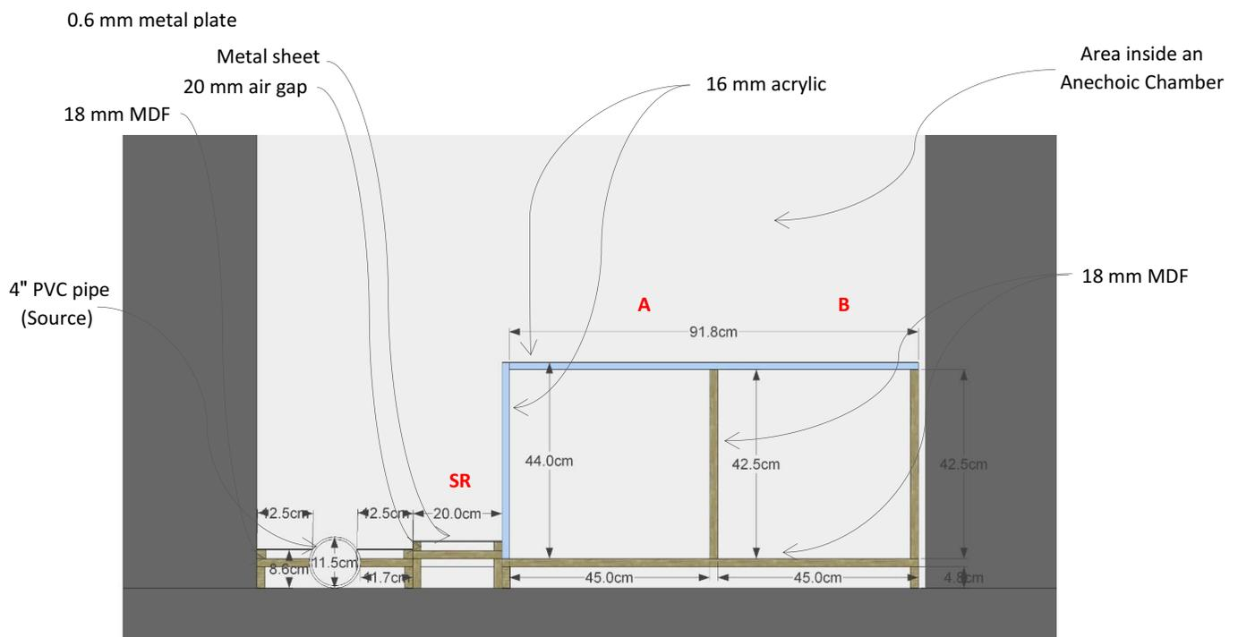
Figure 44: Construction of a 1:10 scale model street-to-roof configuration and Source receiver positions (front elevation).
