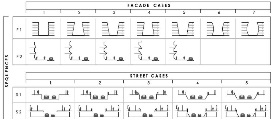
Figure 10: Facade sequences: F1\_General shape of buildings. F2\_Triangular shapes in facades. Street sequences: S1\_Depressed roads at -1.7 m level. S2\_Second level road + parking spaces.
