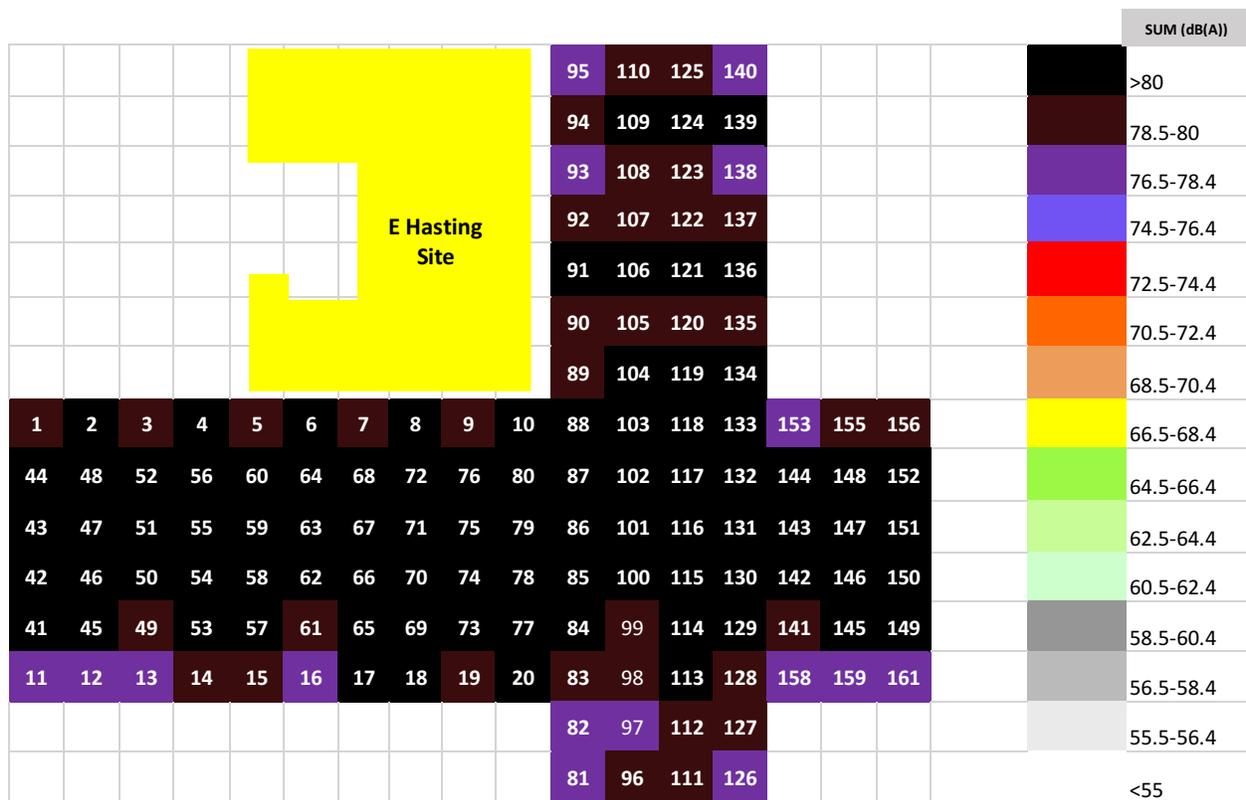
Figure 78: Total dB(A) colored grid response of the street source model analyzed from ASCII output.
