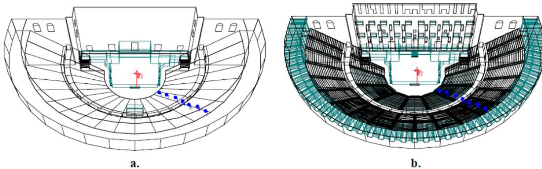
Figure 26: The Aspendos Roman theatre with a performance stage. a. Simple computer model. b. Detailed computer model. The dot on the stage is the source and the dots on the seating area are 7 receiver positions.
