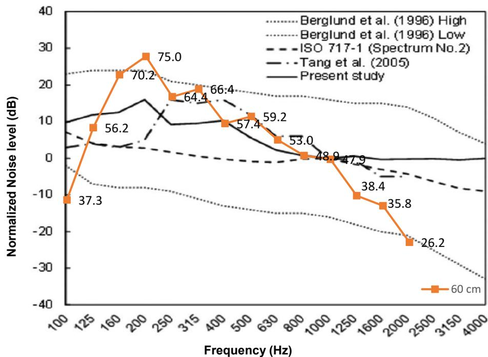
Figure 60: Noise spectra of the source model measured at 60 cm away from the source compared to the traffic spectrums in other studies.
