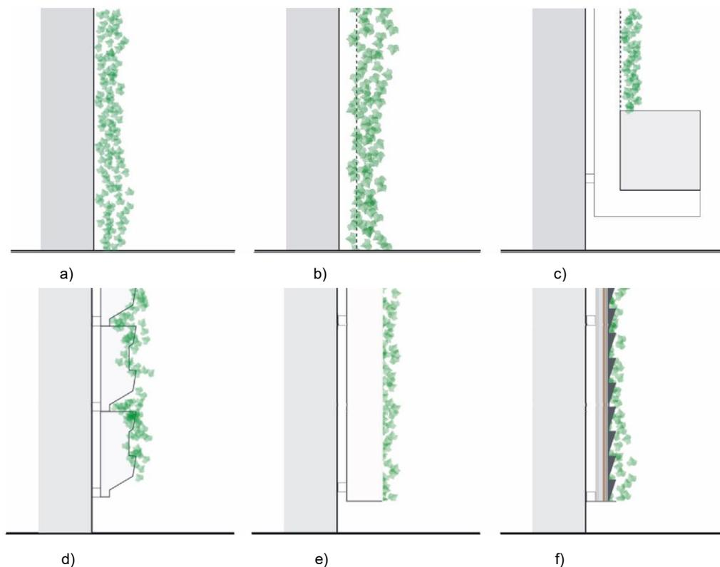
Figure 19: Methods to plant vegetation to the wall: (Perini, K. et al., 2011)
