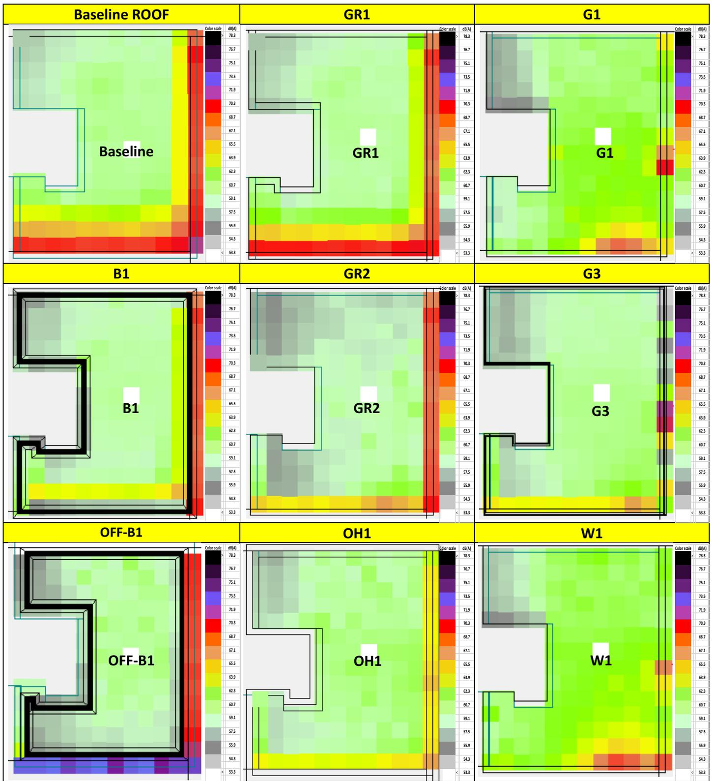
Figure 79: Sonic subzones of the E. Hastings building ROOF and 8 single-design tool configurations on the rooftop.
