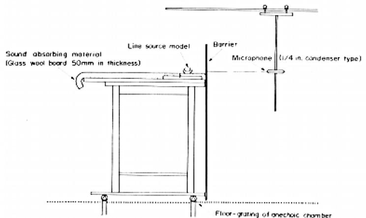
Figure 21: Experiment set-up in an anechoic chamber.
