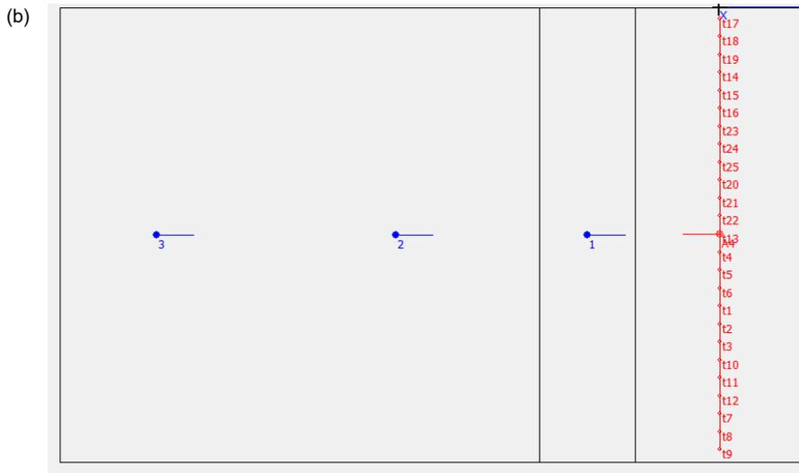
Figure 47: (a) elevation view, (b) plan view of the 25 omni-directional speakers array of the baseline ROOF configuration model in ODEON.
