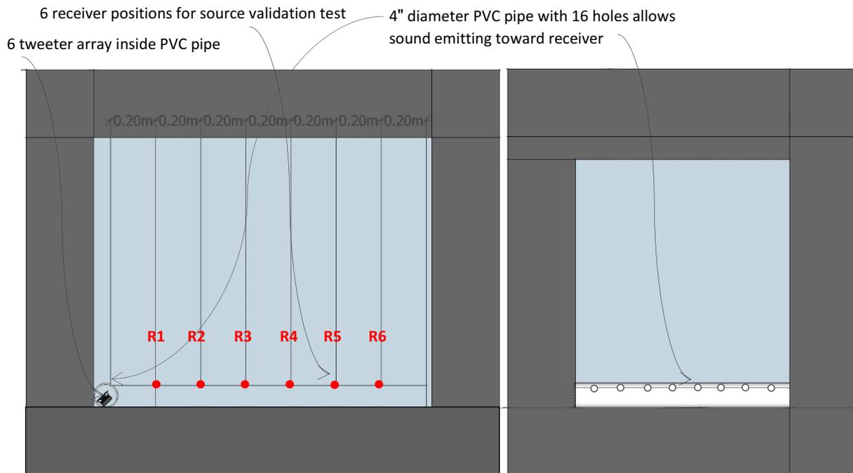
Figures 40-41: Cross-section views of source modelling experiment set-up in the anechoic chamber.
