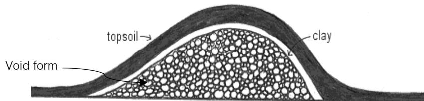
Figure 14: Ideal substrate layers for a berm.
