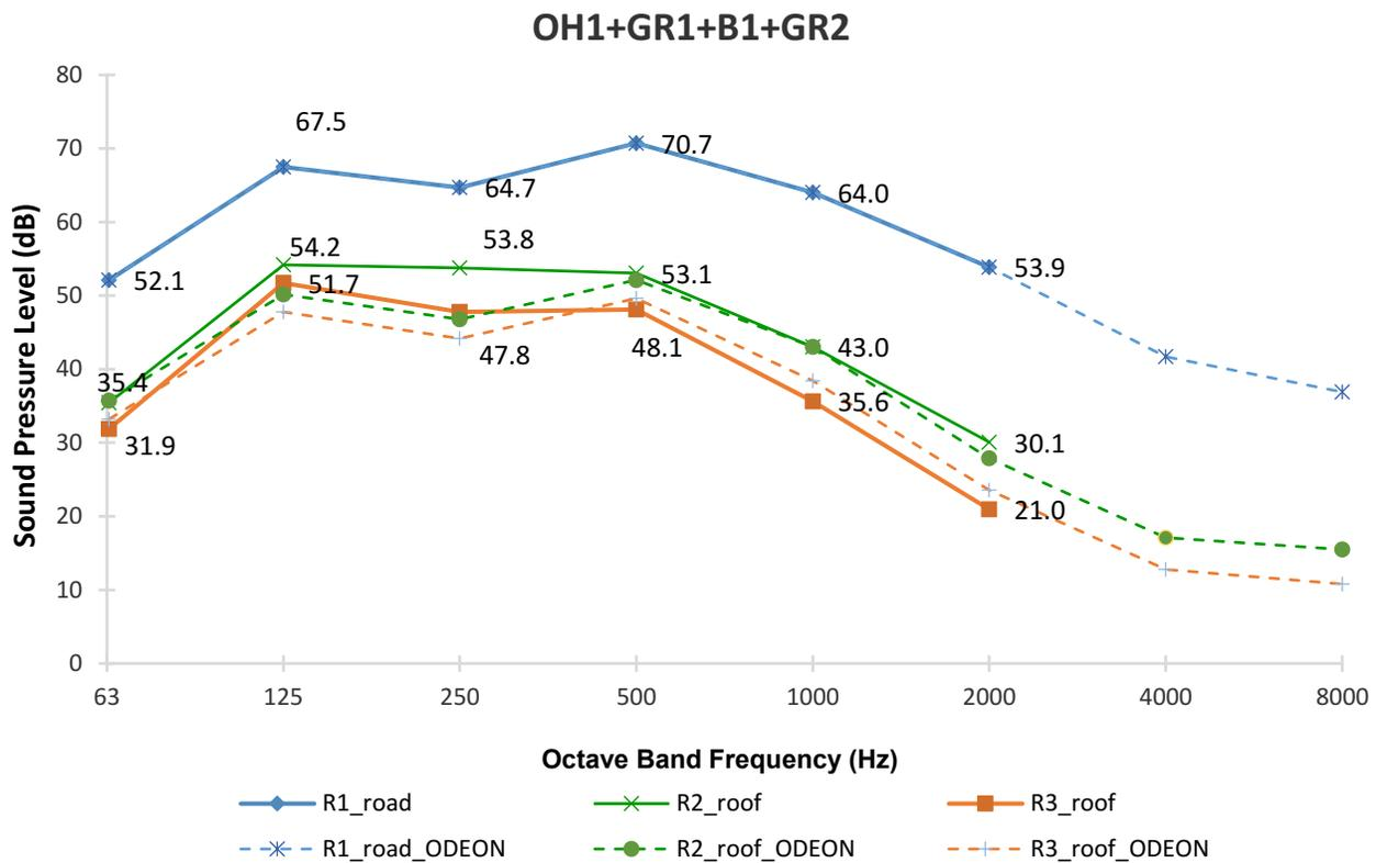
Figure 74: The OH1+GR1+B1+GR2 design tool configuration spectrum analysis.
