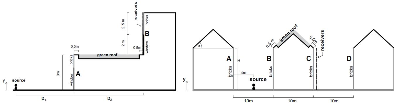
Figure 13: Configuration 1 (left): Green roof on building extension modelled with various substrate depths, Receivers are located along facade B. Configuration 2 (right), Green roof on saddleback roof in various slope angle, Receivers are located along facade C
