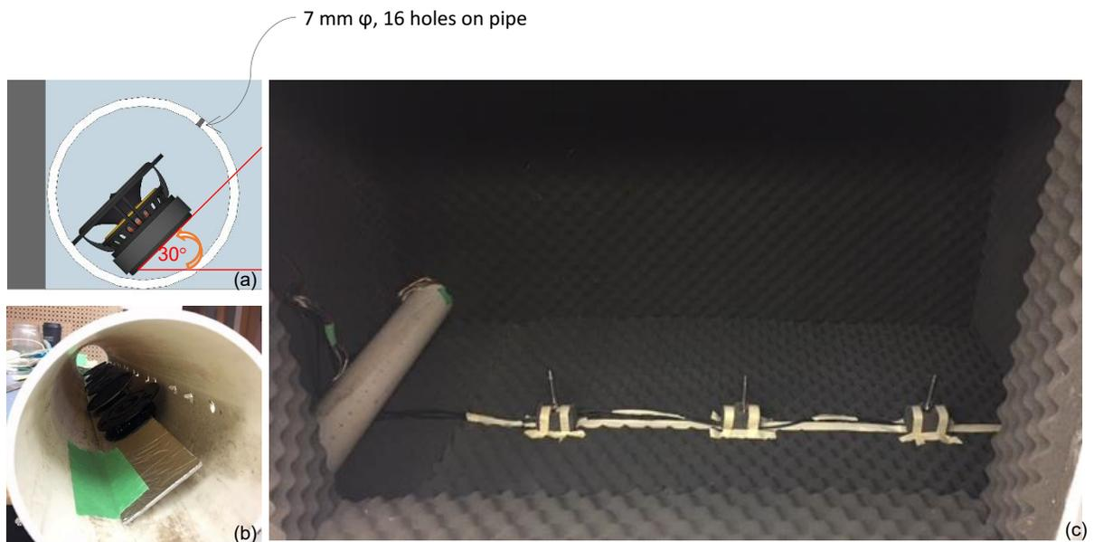
Figure 42: (a) The tweeters angle set-up inside PCV pipe, (b) Image of cross-section of PVC pipe source, (c) Image of line source experiment set-up in anechoic chamber.
