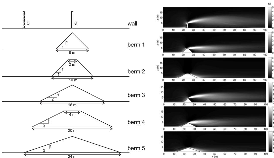
Figure 16: Noise barriers and berm that were numerically evaluated in this study, and the field plots of the vertical gradients in the horizontal component of the wind velocity near the wall and berms. (Van Renterghem and Botteldooren, 2012)
