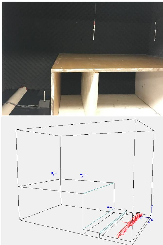
Figure 63: A 1:10 baseline scale model in the AC vs. a baseline simulation model in ODEON.
