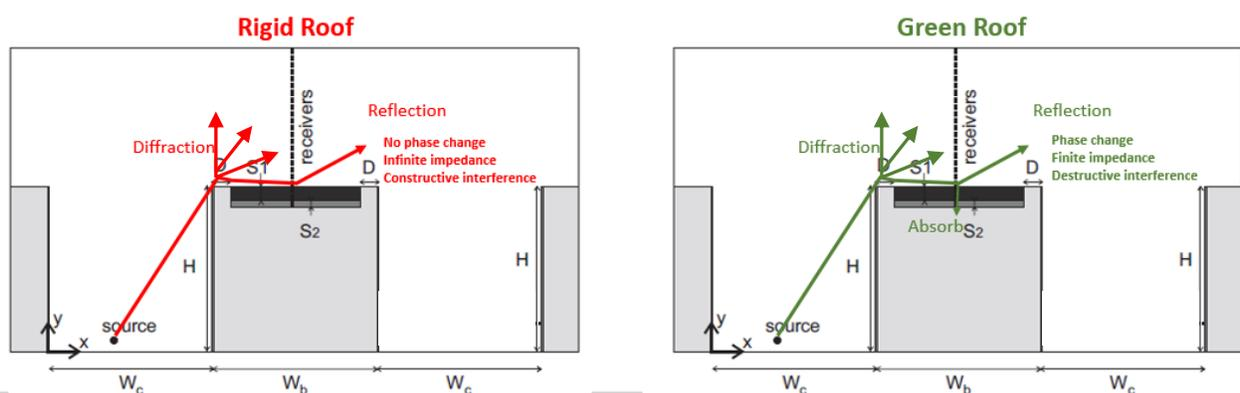
Figure 7: Sound propagation over the green roof in comparison to a rigid roof. (Adopted from Van Renterghem & Botteldooren, 2011)
