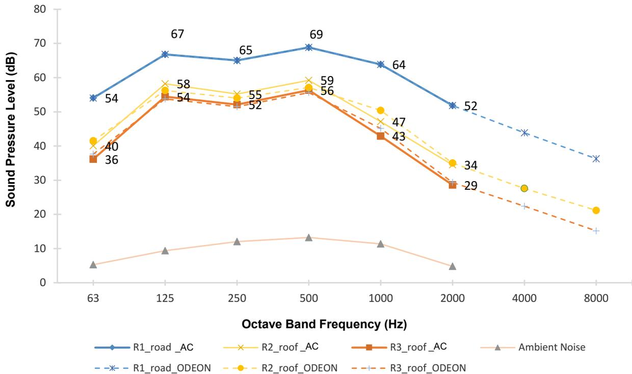
Figure 64: The baseline ROOF configuration spectrum analysis of the 1:10 scale model and ODEON.
