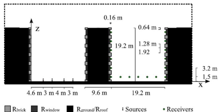
Figure 11: Diagram of 6-storey building over the street canyon set up in the model. (Van Renterghem et al., 2013)
