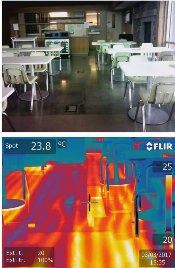
*Figure 54 - Heat distribution within the slab in cafeteria*
