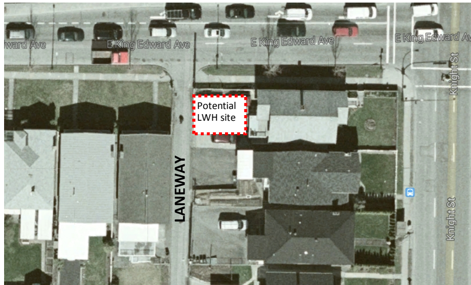
Figure 2: Laneway house site at noisy intersection (Google Earth image). Side yard distance is about 1.5m (5ft) and much narrower than the front yard of 6m (20ft). Both roads have high traffic volume. There is a bus stop on Knight St., which can be both convenient and noisy.
