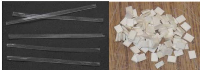
Figure 1: Fibers (Synthetic-L, Cellulose-R).
