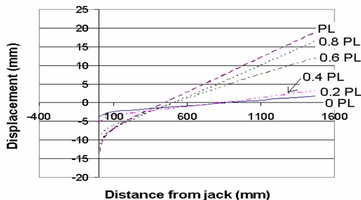
Figure 6: Deflection of Control Slab
