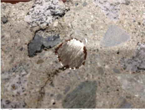
**Figure 9.** Formation of Corrosion Product on corroded rebar.
