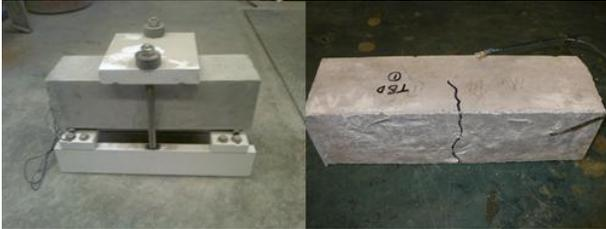
Figure 1. Concrete Specimen under 4 point loading (L) and after being removed from the loading device (R).
