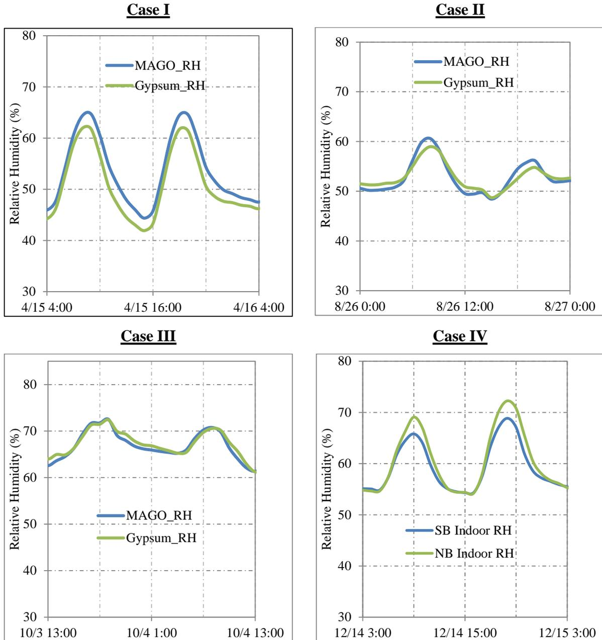
**Figure 17 - Relative humidity comparison of both buildings exposed to high moisture production and normal ventilation rate: (a) Case I (b) Case II (c) Case III (d) Case IV**
