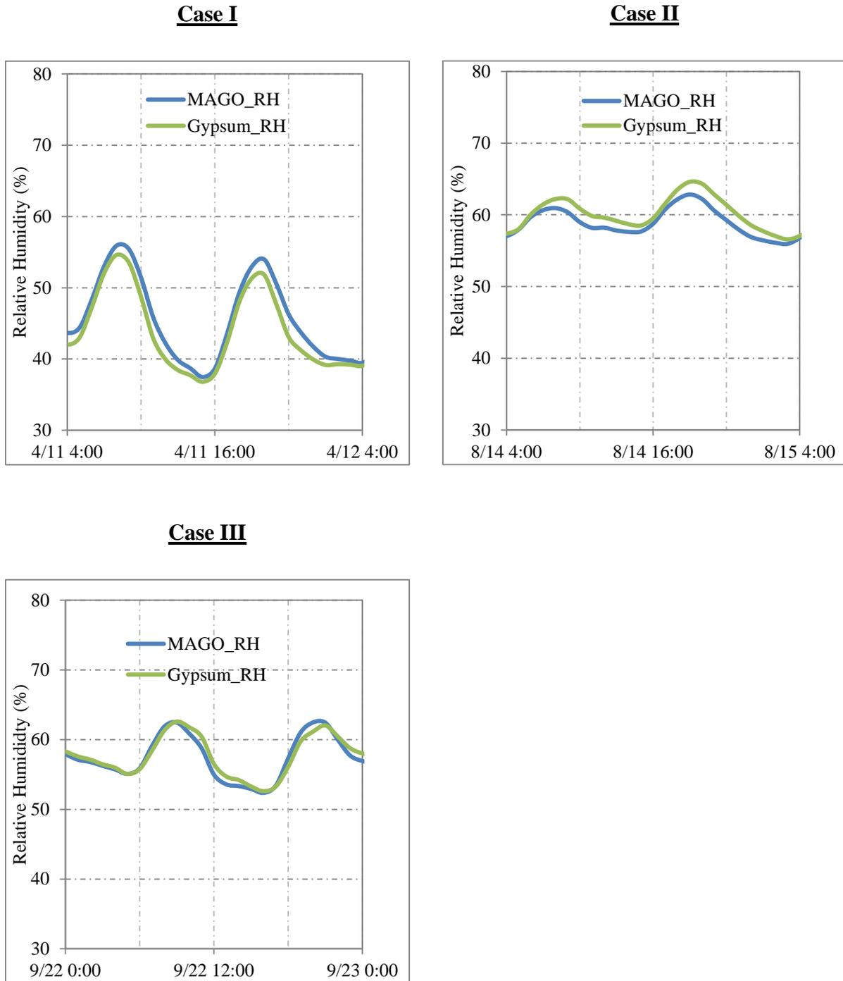
**Figure 15 - Relative humidity comparison of both buildings exposed to normal moisture production and normal ventilation rate: (a) Case I (b) Case II (c) Case III**
