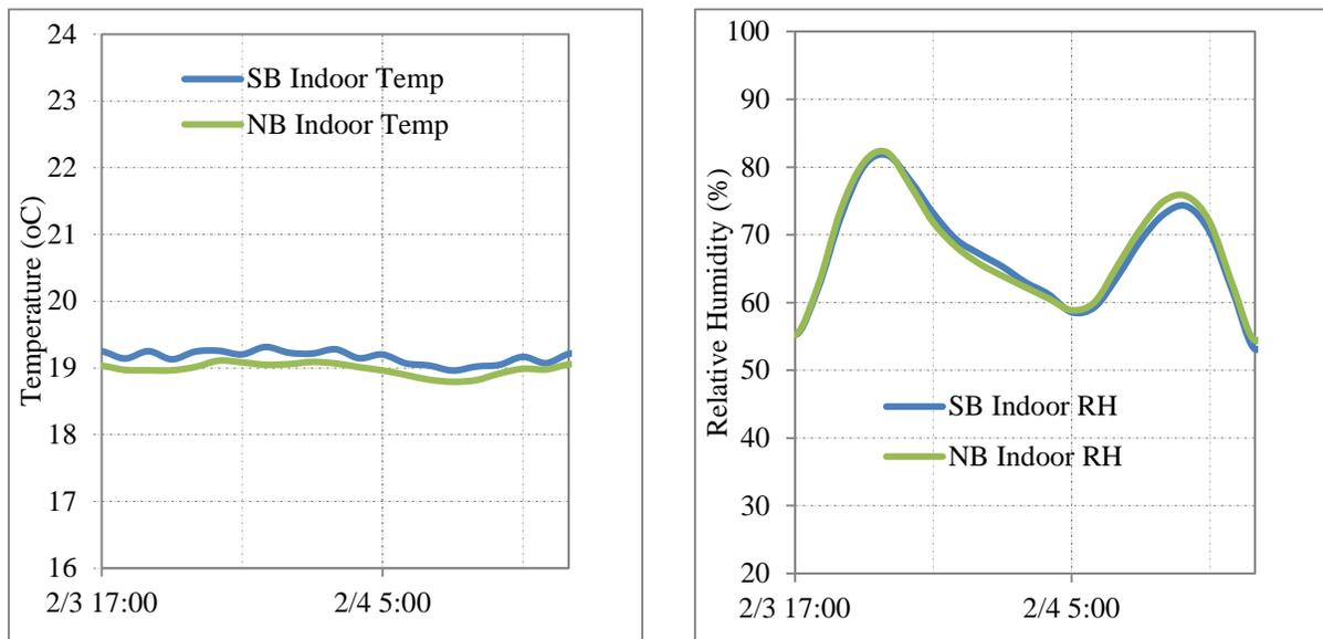
**Figure 12 - Field verification of the moisture production rate in the north and south building: Indoor air temperature (L) and Relative humidity (R) comparison**
