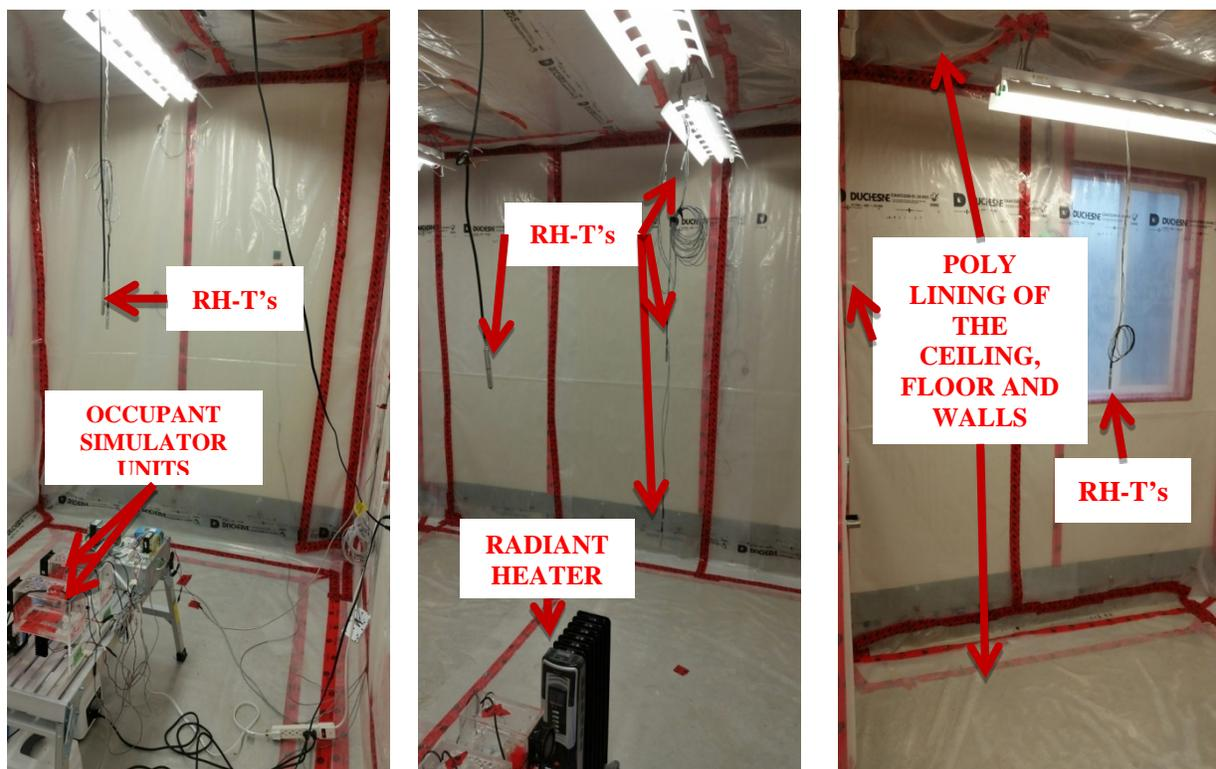
**Figure 9 - Experimental setup of the WBPRP for field verification of the moisture production rates of the occupancy simulators**
