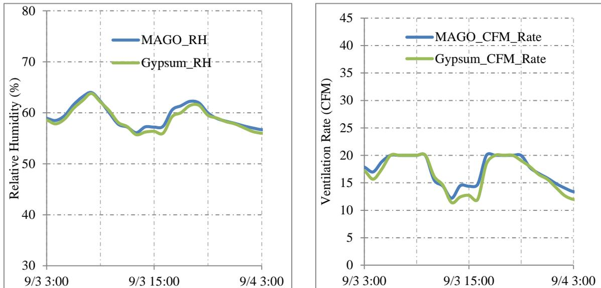
**Figure 19 - Relative humidity (L) and Ventilation rate (R) comparison of both buildings exposed to normal moisture production and relative humidity controlled ventilation rate (Unpainted)**
