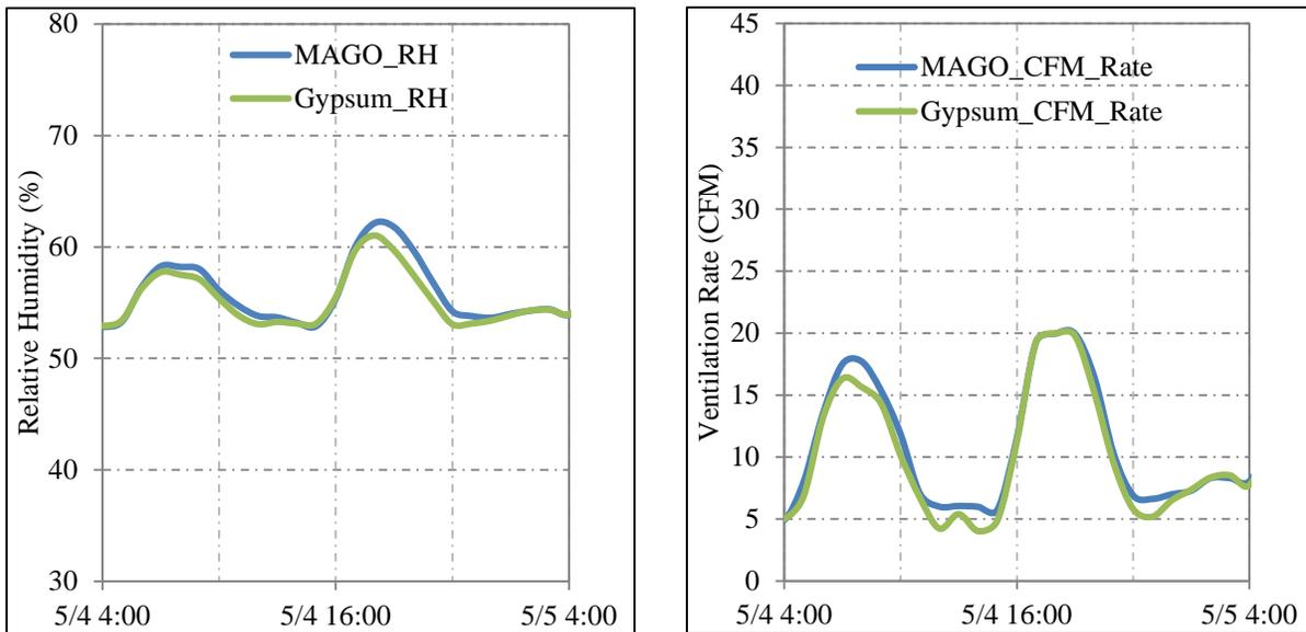
**Figure 18 - Relative humidity (L) and Ventilation rate (R) comparison of both buildings exposed to normal moisture production and relative humidity controlled ventilation rate (Painted)**
