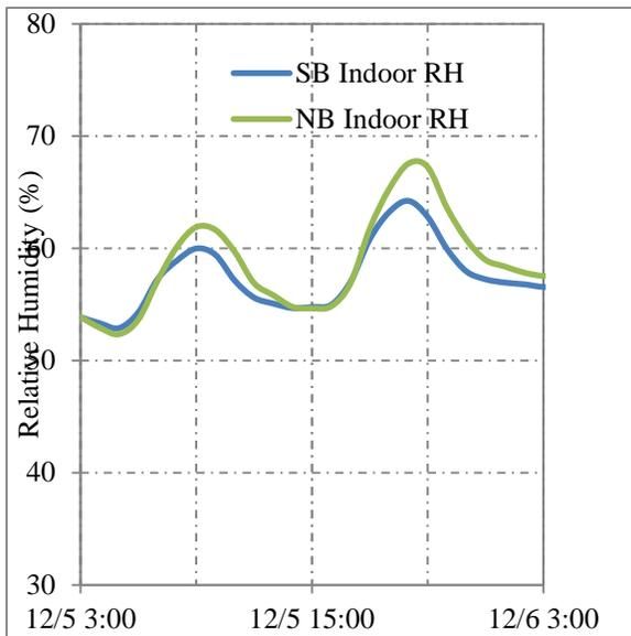
**Figure 16 – Relative humidity of north and south buildings exposed to normal moisture production and low ventilation rate: (a) Case I (b) Case II (c) Case IV**
