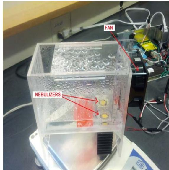
**Figure 3 - Laboratory setup for calibration of the indoor simulation units[34]**
