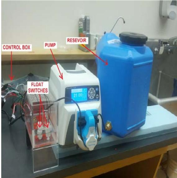
**Figure 1 - Humidification System Components of the occupant simulator system [34]**
