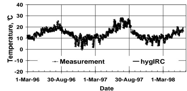
Figure 13 Comparison of measured and computed temperature at the middle section
