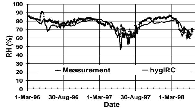
Figure 8 Comparison of measured and computed relative humidity at the outer section
