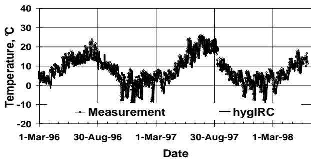
Figure 14 Comparison of measured and computed temperature at the outer section
