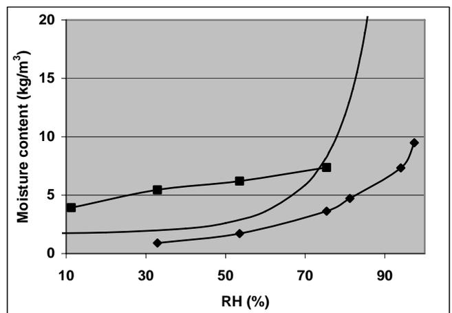
Figure 4 Sorption isotherm of Aerated concrete
