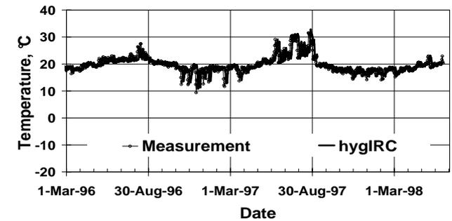
Figure 12 Comparison of measured and computed temperature at the inner section
