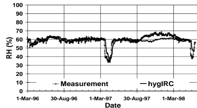
Figure 9 Relative humidity comparison with modified indoor relative humidity at the inner section
