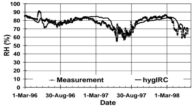
Figure 11 Relative humidity comparison with modified indoor relative humidity at the outer section
