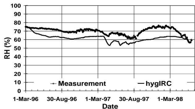
Figure 7 Comparison of measured and computed relative humidity at the middle section
