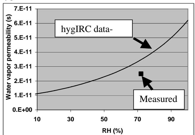
Figure 5 Water vapor permeability of Aerated concrete
