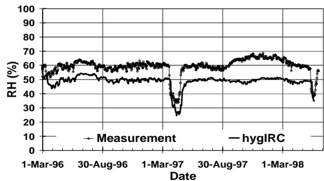
Figure 6 Comparison of measured and computed relative humidity at the inner section
