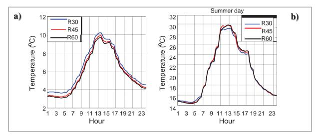
Figure 5 Attic air temperature for different insulation during winter (a) and summer (b) days
