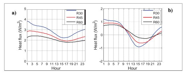
Figure 6. Total heat flow during winter (a) and summer (b) for different attic insulation cases
