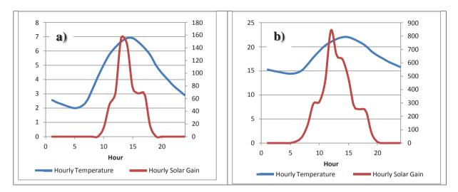
Figure 1 Hourly temperature and solar radiation during a) Winter and b) Summer typical days
