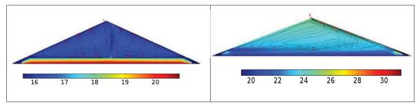
Figure 2 (a) and (b) Airflow distribution in attic space for cases without solar gain and with solar gain
