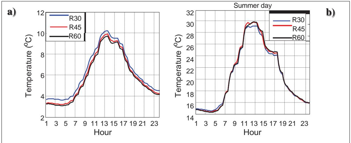
Figure 5 Attic air temperature for different insulation during winter (a) and summer (b) days
