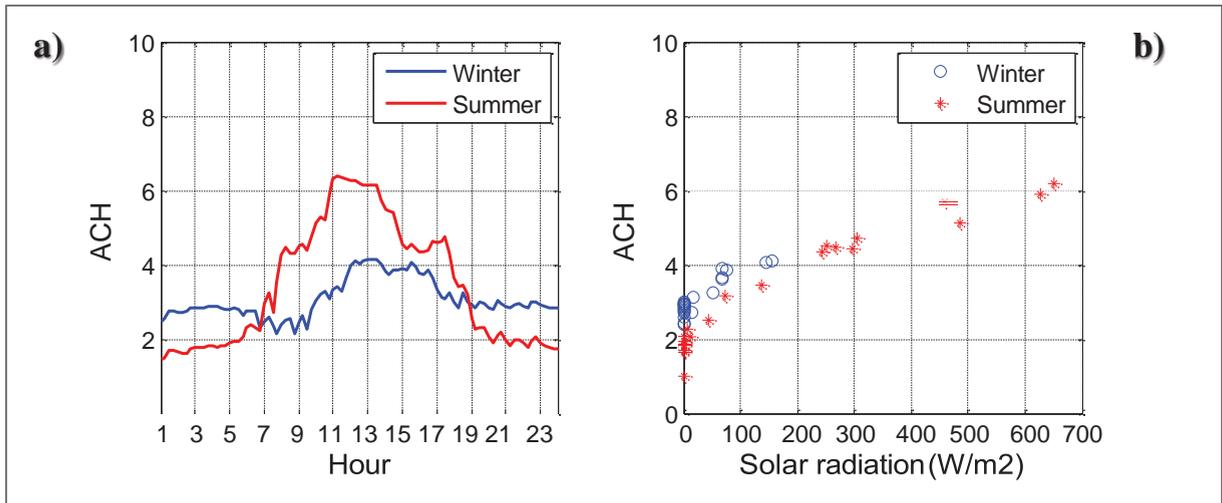
Figure 3 Attic ventilation rates during a typical winter and summer days (a); and ACH vs solar radiation (b)
