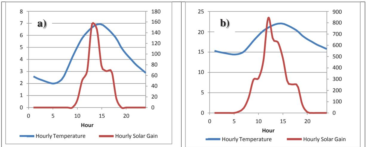
Figure 1 Hourly temperature and solar radiation during a) Winter and b) Summer typical days
