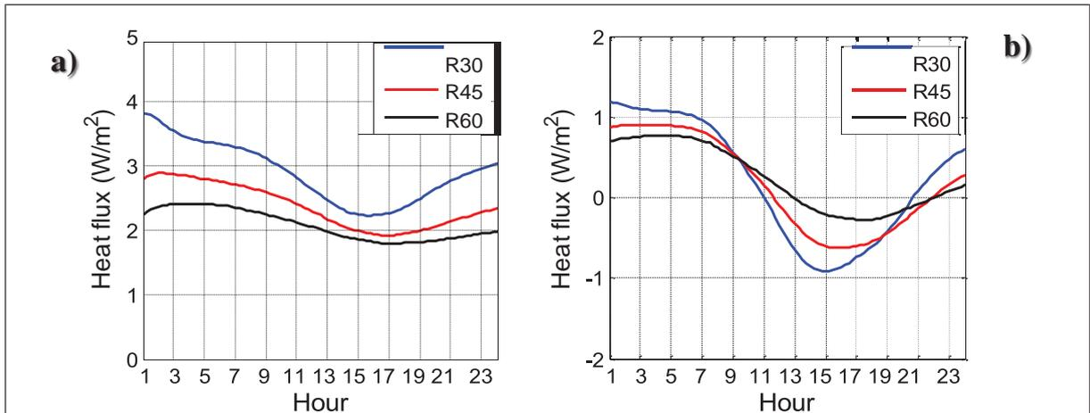
Figure 6. Total heat flow during winter (a) and summer (b) for different attic insulation cases
