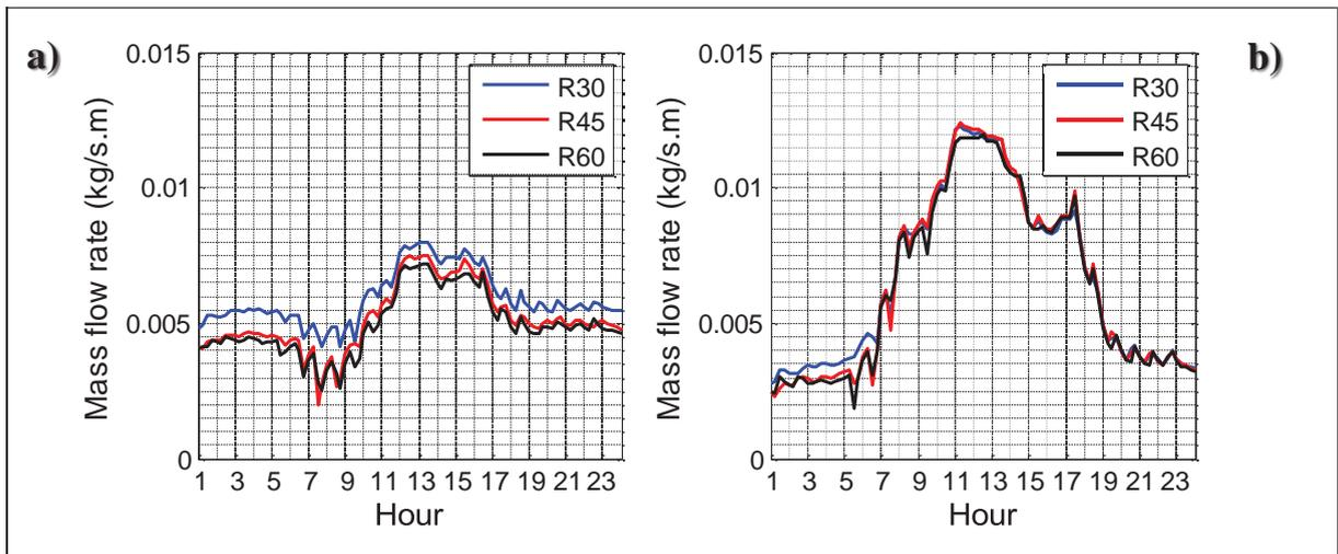
Figure 4 Attic ventilation rates during a typical winter (a) and summer (b) days
