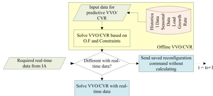
Fig. 3. Predictive part of offered VVO/CVR Engine
