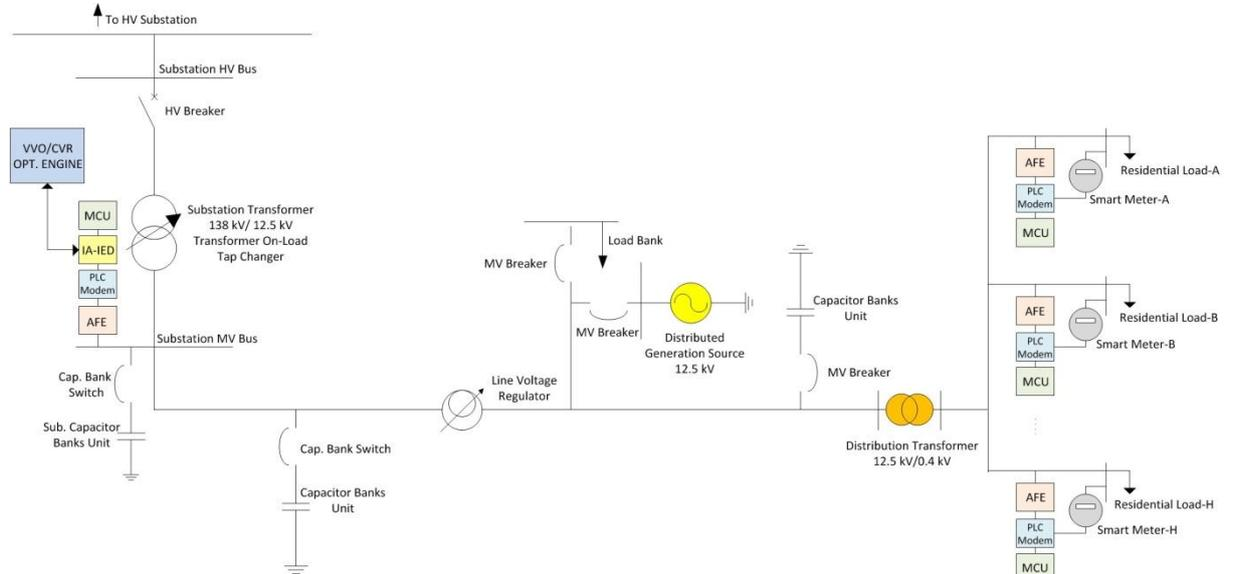
Fig. 1. Main structure of proposed approach for VVO/CVR for a distribution feeder
