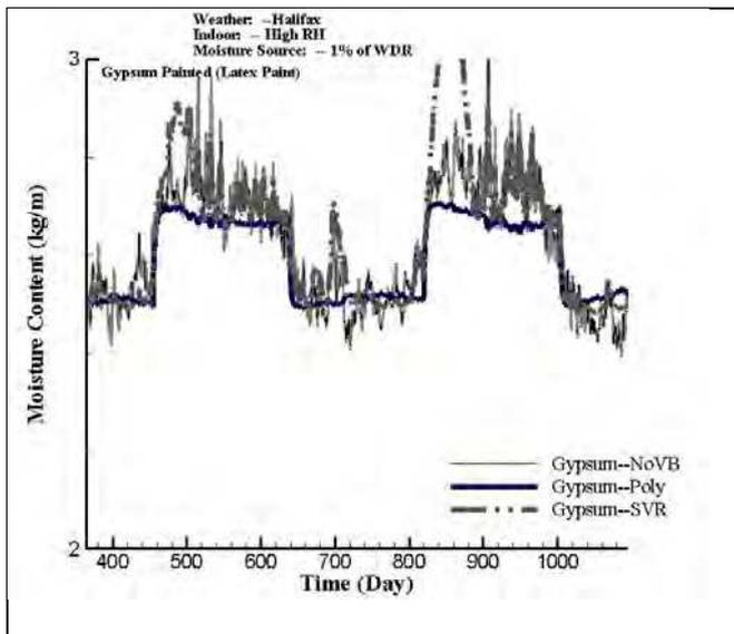
**Figure 7** – Bulk Moisture content (kg/m) of interior gypsum board in relation to time (day) for simulations on wall assemblies having different vapour control strategies with 1% WDR and interior finish painted with latex paint.
