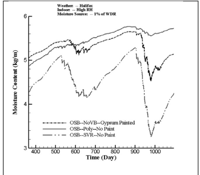
**Figure 5** – Bulk Moisture Content (kg/m) of OSB versus time (day) for simulations on wall assemblies having different vapour control strategies with 1 % WDR and interior finish unpainted or painted with acrylic paint in the case of No VB.
