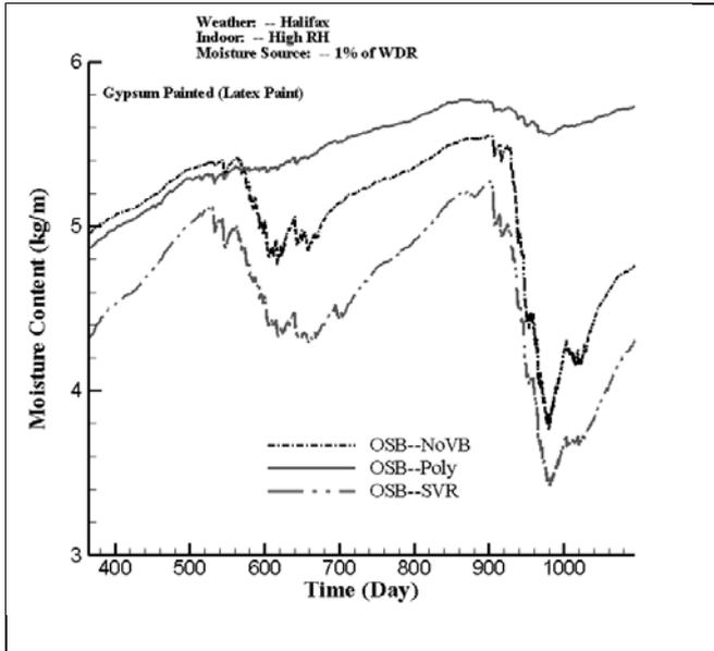
**Figure 3** – Bulk Moisture Content (kg/m) of OSB versus time (day) for simulations on wall assemblies having different vapour control strategies with 1 % WDR and interior finish painted with latex paint
