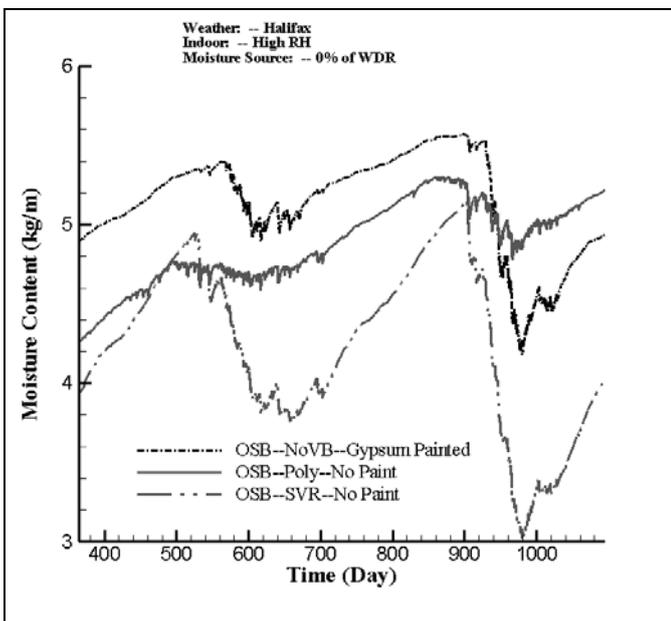
**Figure 4** – Bulk Moisture Content (kg/m) of OSB versus time (day) for simulations on wall assemblies having different
