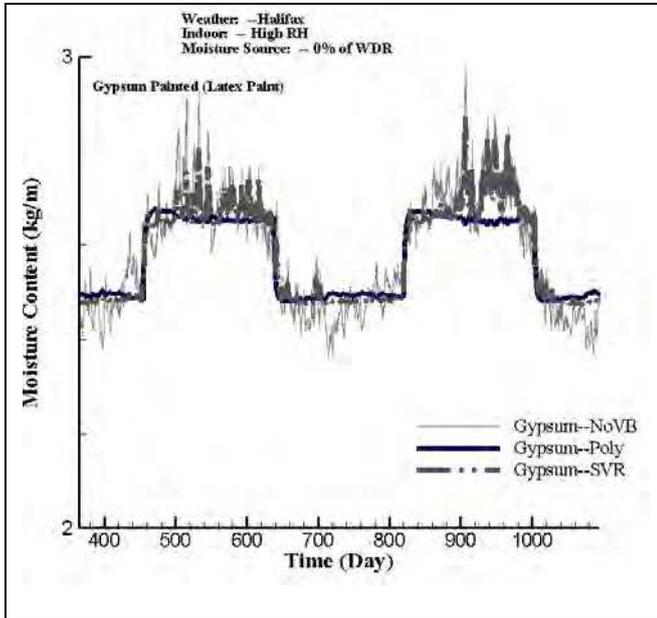
**Figure 6** – Bulk Moisture content (kg/m) of interior gypsum board in relation to time (day) for simulations on wall assemblies having different vapour control strategies with 0% WDR and interior finish painted with latex paint.
