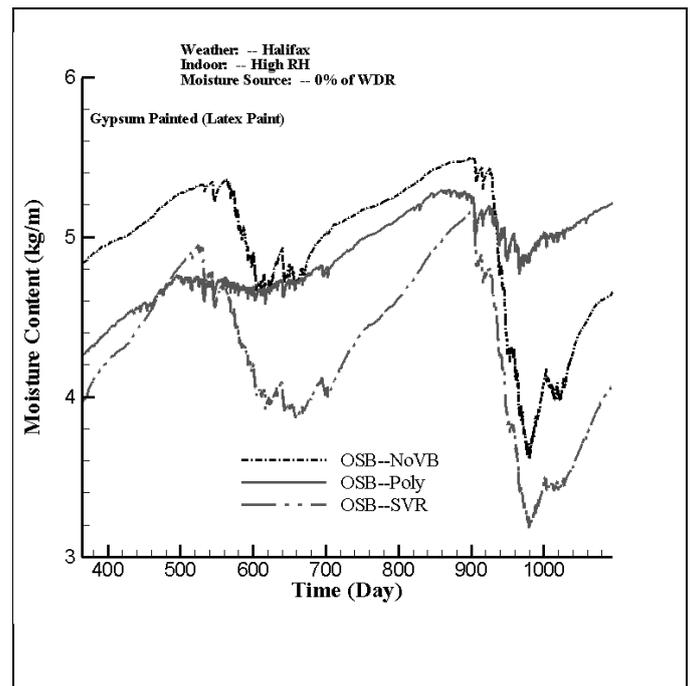
**Figure 2** – Bulk Moisture Content (kg/m) of OSB versus time (day) for simulations on wall assemblies hav-
