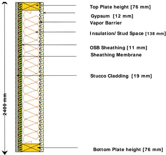
**Figure 1** – Wall Configuration
