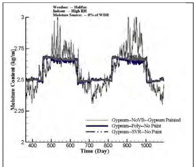
**Figure 8** – Moisture content (kg/m) of interior gypsum board in relation to time (day) for simulations on wall assemblies having different vapour control strategies with 0% WDR and interior finish unpainted.
