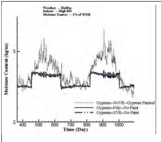
**Figure 9** – Moisture content (kg/m) of interior gypsum board in relation to time (day) for simulations on wall assemblies having different vapour control strategies with 1% WDR and interior finish unpainted
