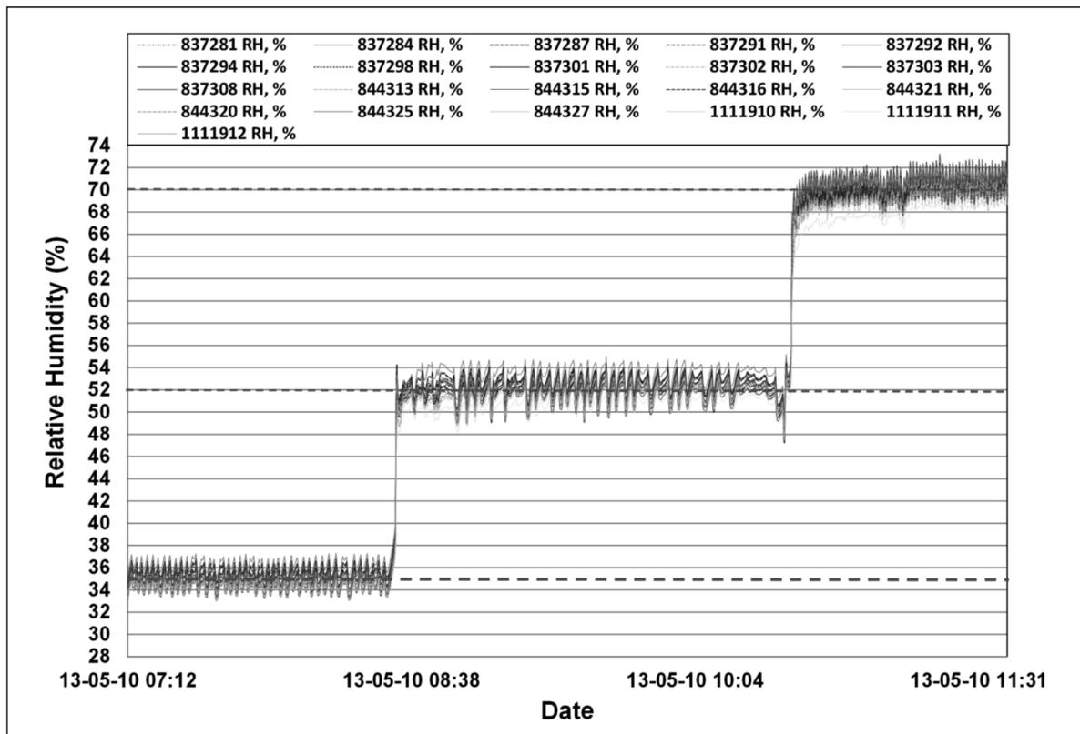
FIGURE 1: RELATIVE HUMIDITY READINGS OF HOBO DATA LOGGERS DURING THE CALIBRATION PROCESS.
