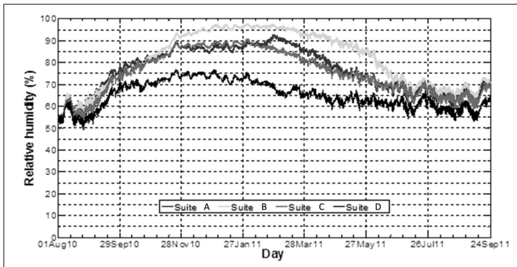
**FIGURE 6: RELATIVE HUMIDITY OF EXTERIOR GYPSUM LAYER AT THE INTERIOR SURFACE FOR FOUR SUITES.**
