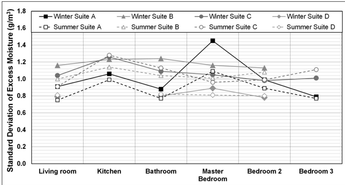
FIGURE 5: STANDARD DEVIATION OF EXCESS HUMIDITY VARIATIONS IN THE TWENTY-TWO ROOMS DURING THE WINTER AND SUMMER PERIODS.
