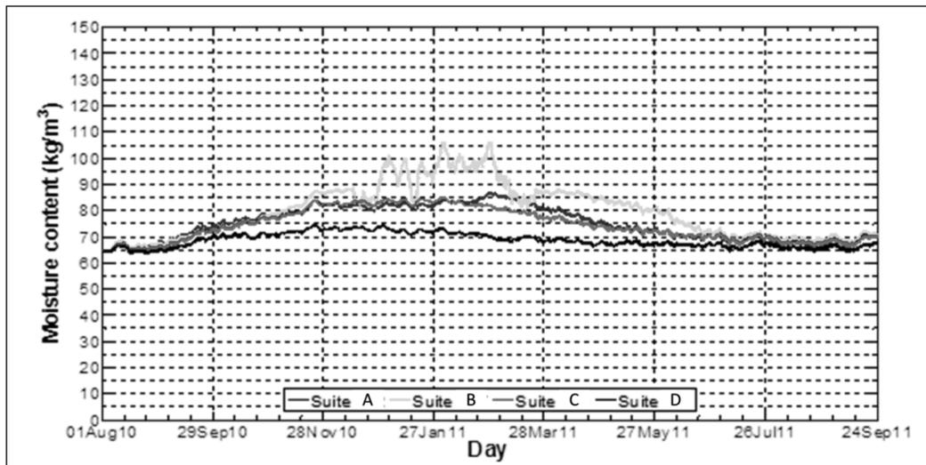
**FIGURE 7: EXTERIOR GYPSUM LAYER MOISTURE CONTENT FOR FOUR SUITES.**
