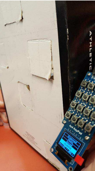
Figure 13: OLED display showing three latched sensors in alarm mode, with the makeshift windows closed to illustrate the latch.
