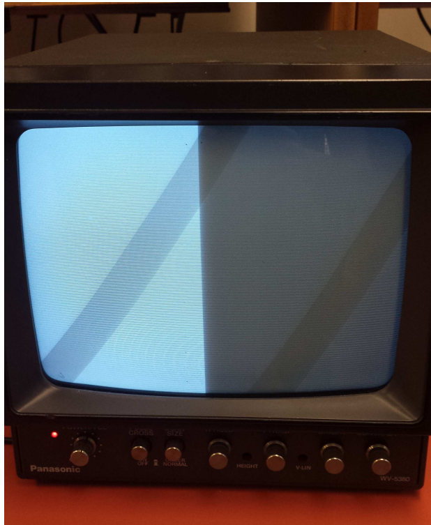
Figure 4: Demonstration Setup. Note: Grey diagonal bars are caused due to differences in the frame rate of the display and the shutter rate of the camera. The display is in fact half white and black.
