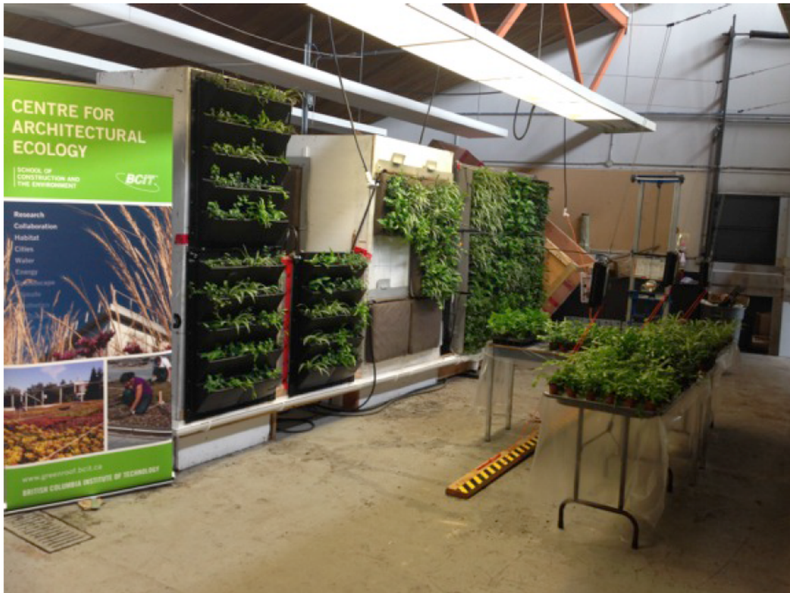
Figure 32. Preparation phase at the Center for Architectural Ecology (BCIT). The living wall panels were developed as joint experiment set-up with Ivan Cheung (UBC, The impact of living walls on indoor air quality).
