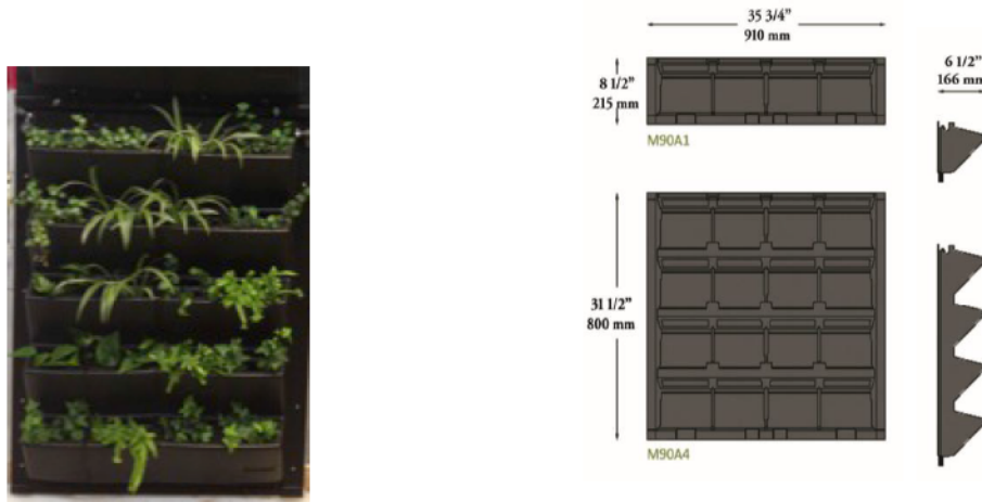
Figure 25. interior living wall system dimension. (Carrier Type A)
