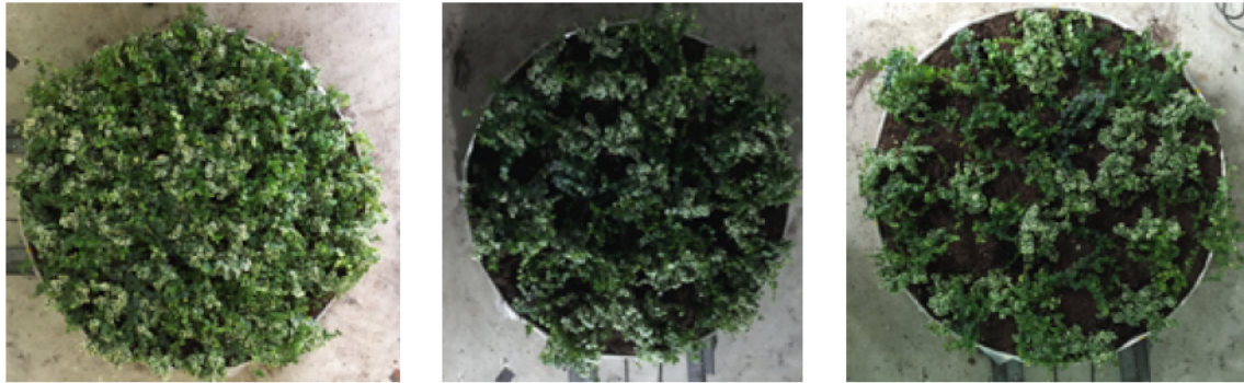
Figure 68. The measurement condition of 100 mm substrate with Creeping Fig. (a) 25% vegetation coverage, (b) 50% vegetation coverage, (c) 100% vegetation coverage
