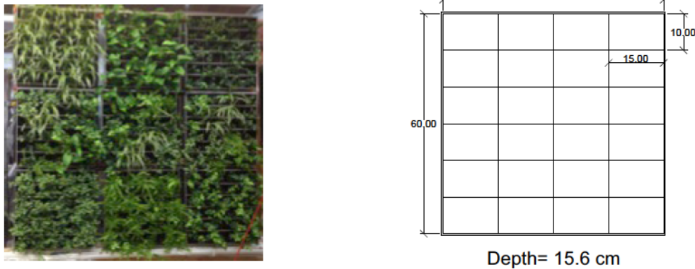
Figure 26. interior living wall system. (Carrier Type B)
