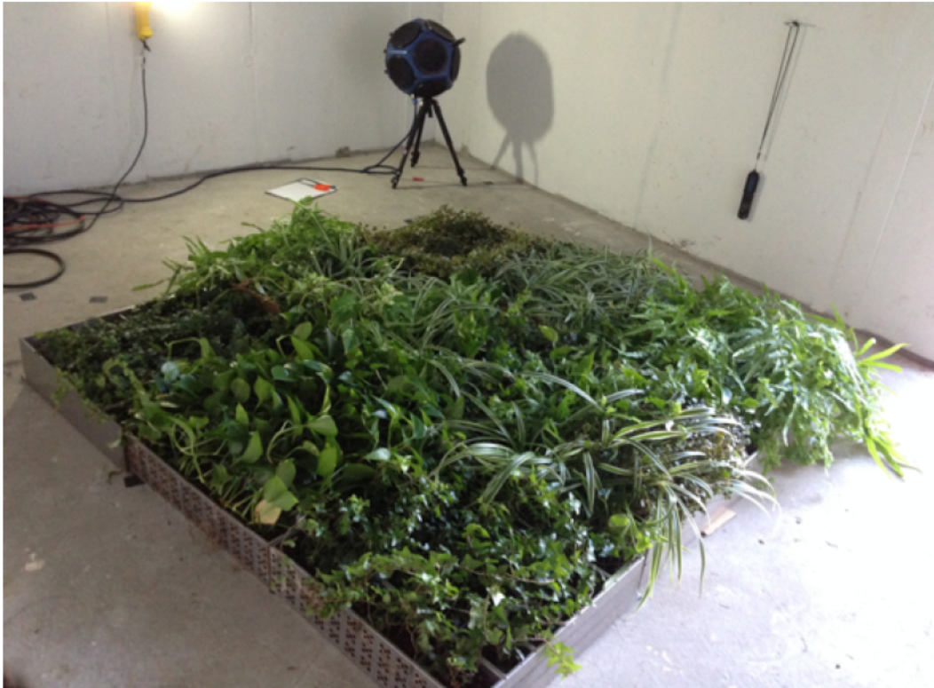
Figure 57. The measurement condition of the living wall made of 8 vegetated Carrier B panels
