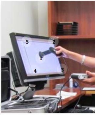
Figure 3. UnforsXi Light Detector Measuring 5 Areas of Monitor
