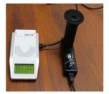
Figure 2. Light Detector without (left) and with (right) luminance tube
