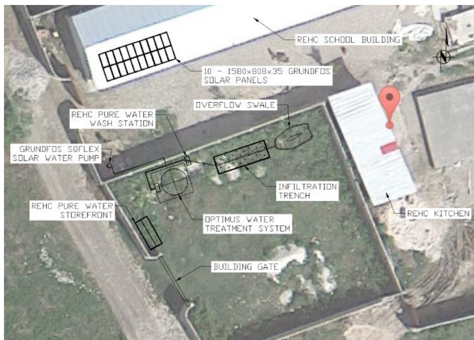
Figure 2: Plan view of water filtration system component layout on site (Google, 2015)
