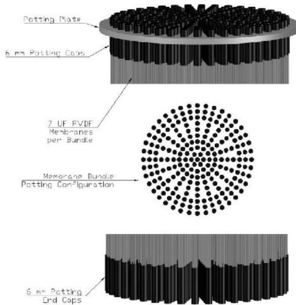
Figure 10: Membrane fibre potting configuration
