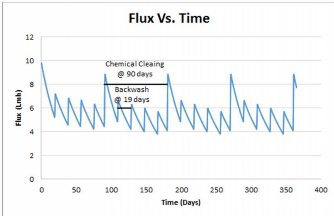
Figure 12: Optimized Backwash and Cleaning Cycle
