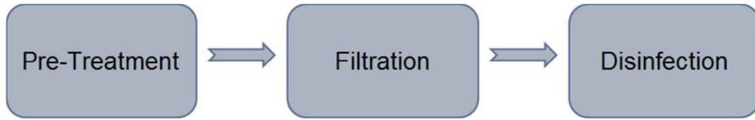
Figure 4: Direct filtration process model
