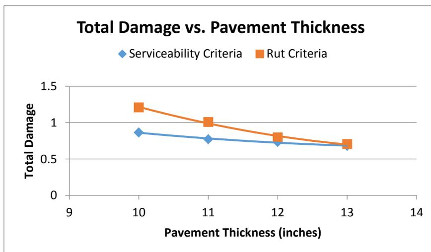
Figure 22: Total damage vs. pavement thickness (Kim, 2015)
