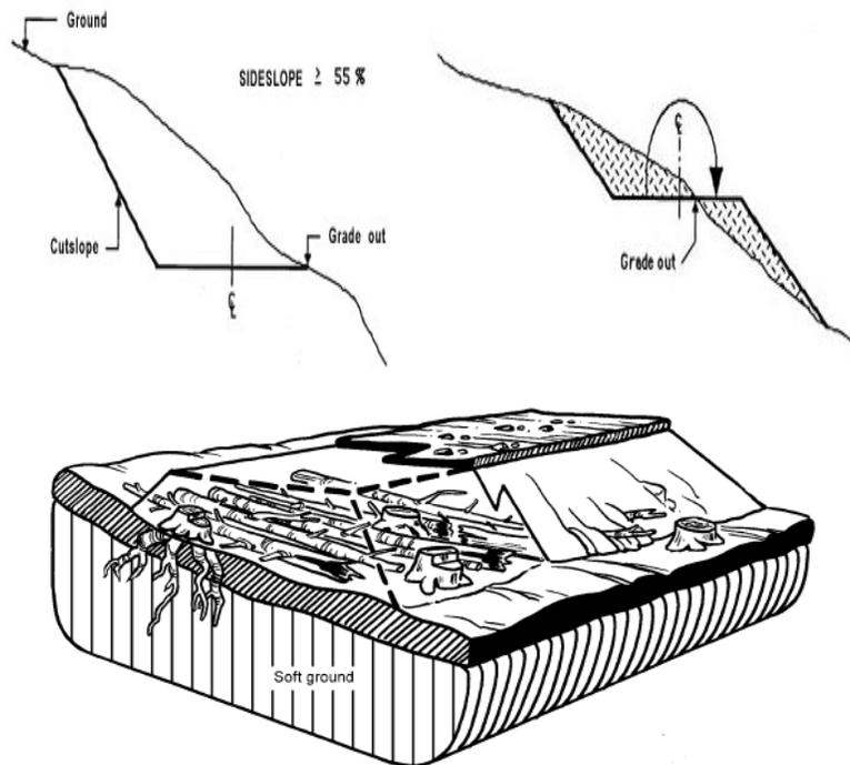
Figure 16: Full-benching (top left), self-balancing (top right), over-landing (bottom) design (Ministry of Forests, Lands and Natural Resource Operations, 2013)
