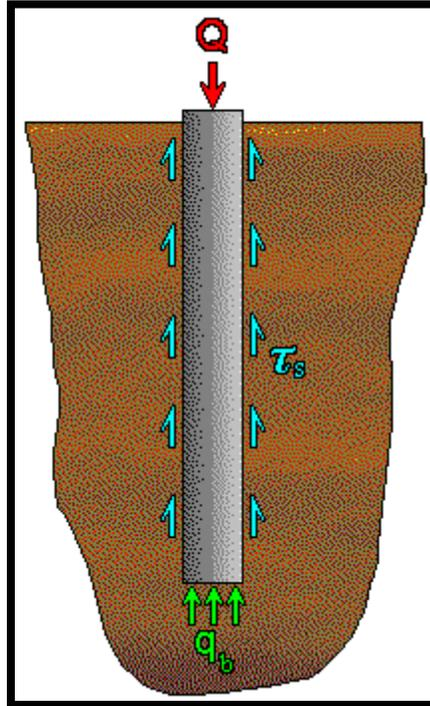
Figure 42: Forces on a friction pile (environment.uwe)
