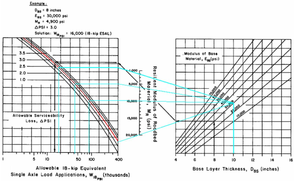
Figure 20: Design chart considering allowable serviceability loss (AASHTO, 1993)
