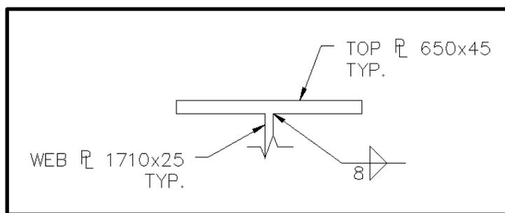
Figure 41: Upper portion of plate girder cross section (Ip, 2015)
