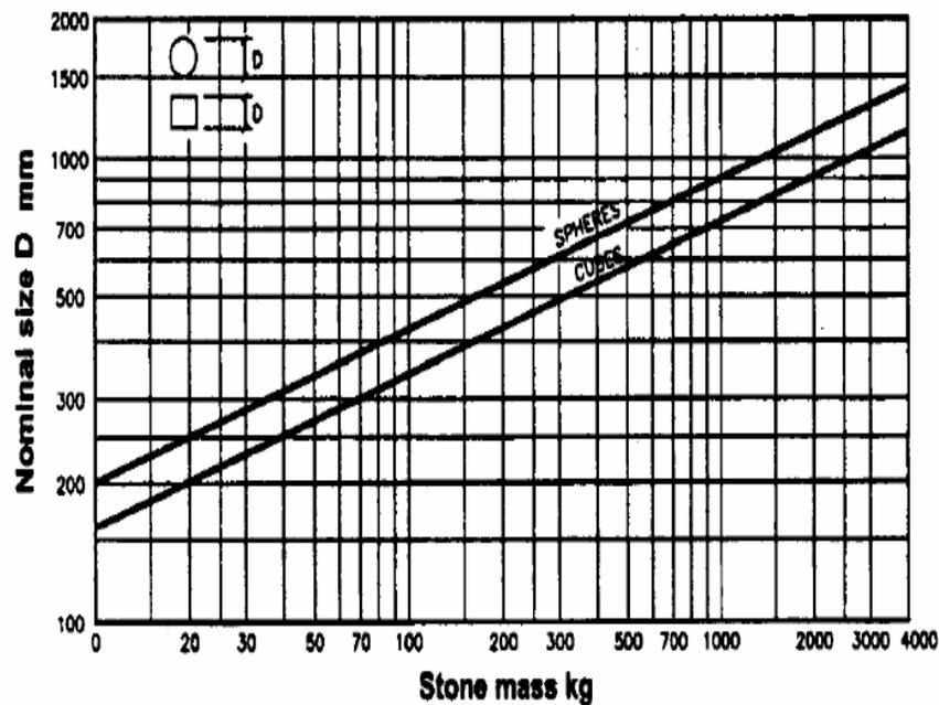
Figure 49: Riprap size and weight for a specific weight of 2.65 (Ministry of Transportation and Highways, 1999)
