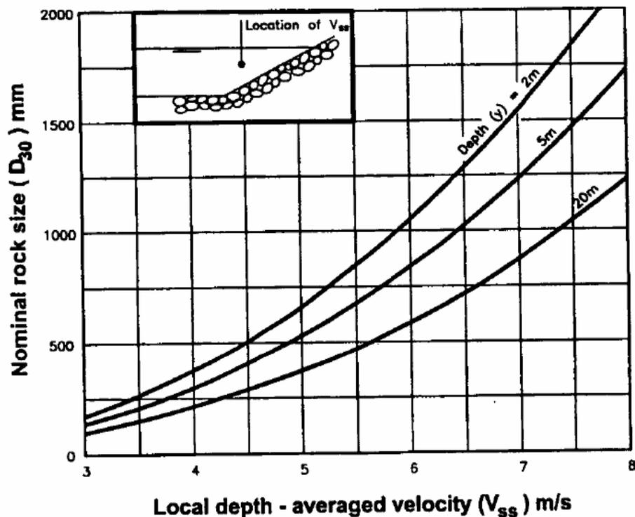
Figure 48: Required rock sizes for a range of velocities and depths (Ministry of Transportation and Highways, 1999)
