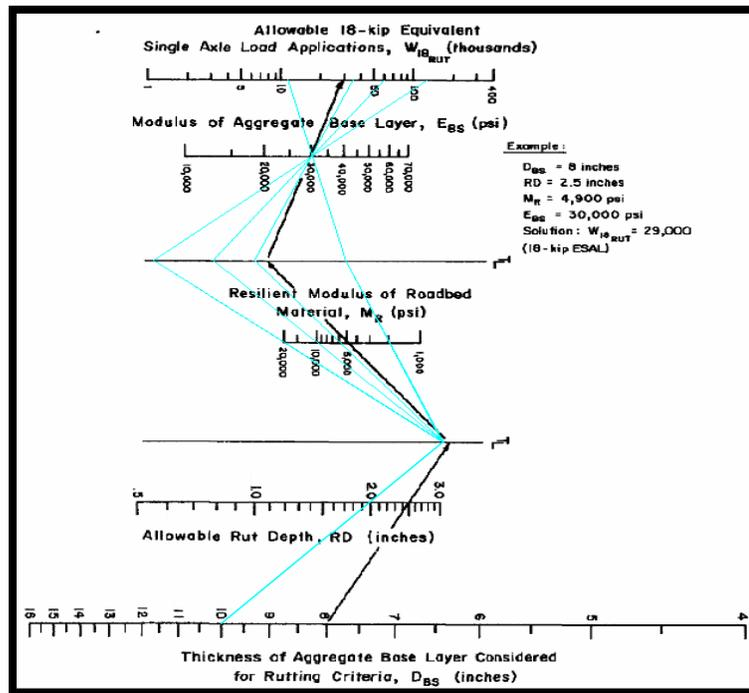
Figure 21: Design chart considering allowable rutting (AASHTO, 1993)
