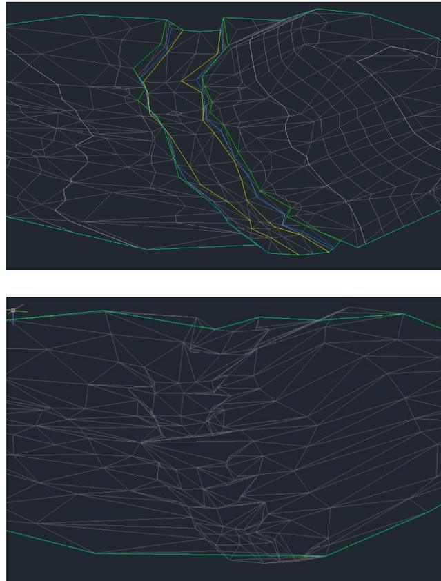
Figure 5: Site 10 Processed surface model (above) unprocessed (below) (Kim, 2015)
