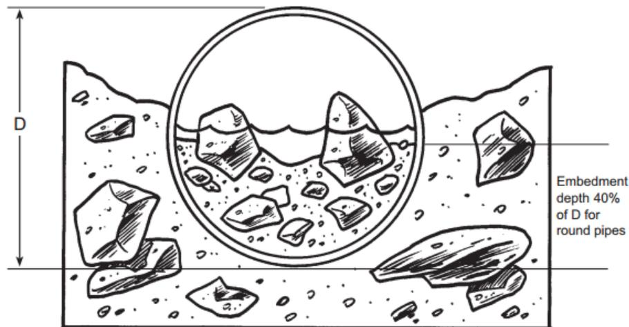
Figure 44: Culvert embedment depth (Ministry of Environment, 2012)
