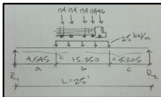
Figure 37: Option A L-100 truck location where max moment induced (Ip, 2015)
