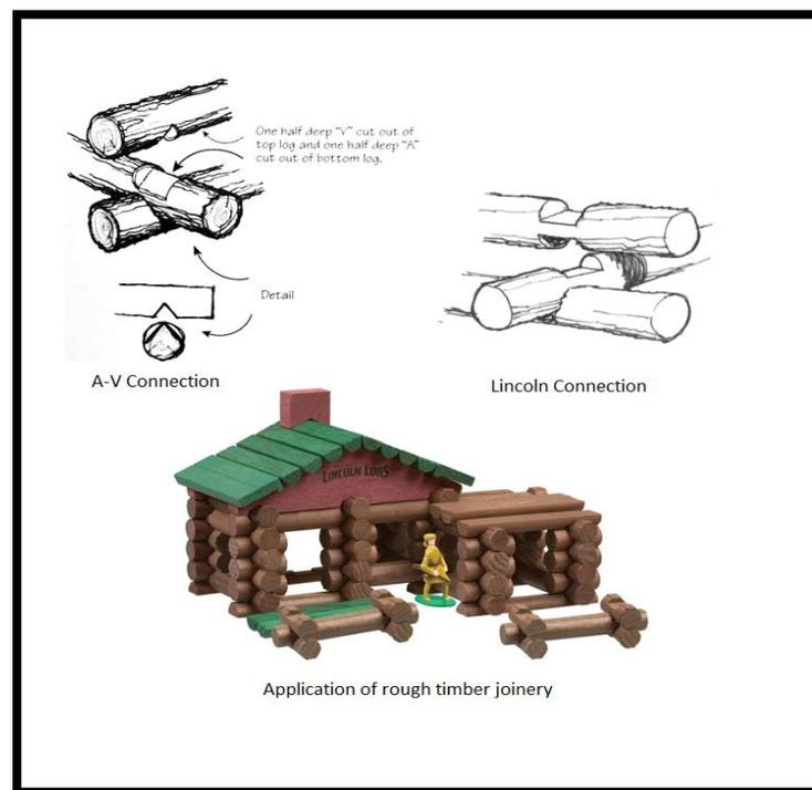
Figure 29: Lincoln and A-V connection detail and application (woodlandia, 2006)
