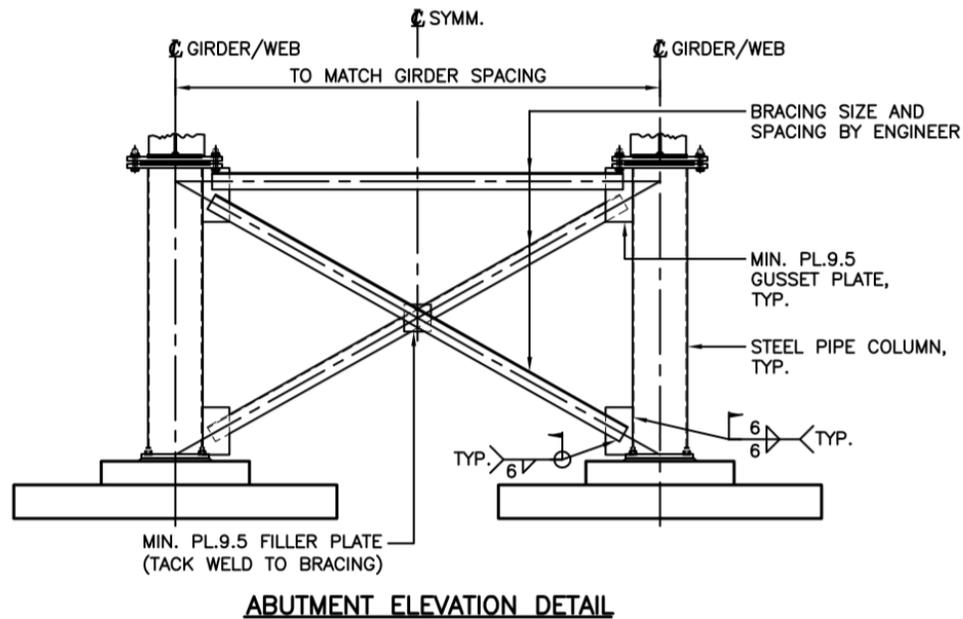
Figure 43: Bearing pad foundation with pile stilts (MFLNRO, n.d.)
