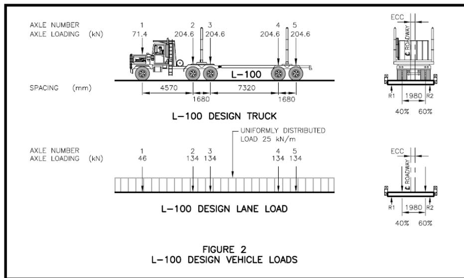
Figure 34: L-100 design vehicle loads (MFLNRO, n.d.)
