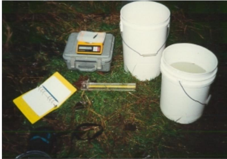
Figure 8. Fish Sampling Equipment
