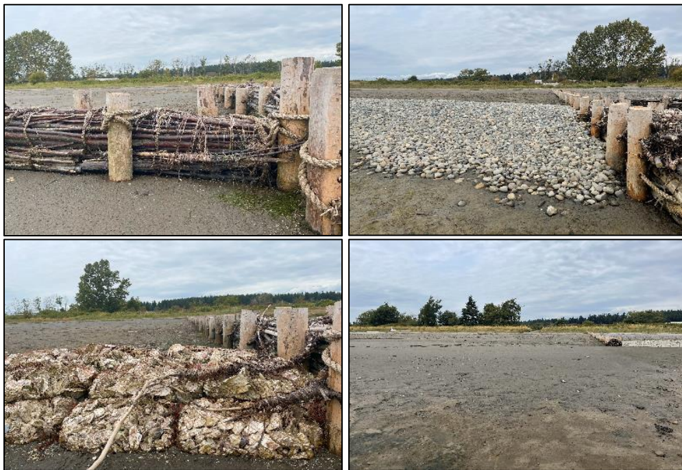
Figure 6: Image showing the four edge treatments at the S1 LDPP study site in Boundary Bay, British Columbia. Clockwise from the top left: brushwood dam, gravel berm, sand berm, oyster bag berm.
