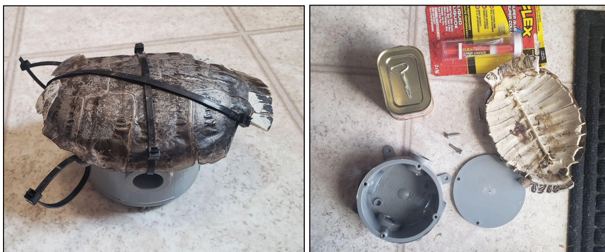
Figure 8. Artificial turtle carcass constructed from a turtle shell and a Carlton conduit body junction box. The artificial turtle carcass was used to estimate the number of turtle road mortalities removed between surveys at Baynes Lake, BC during the summer of 2023.
