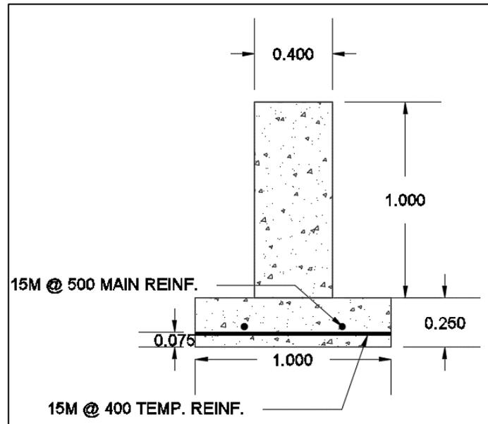
Figure 15: Strip Footing Foundation (See Volume II, 'Footing Plan - Section B')
