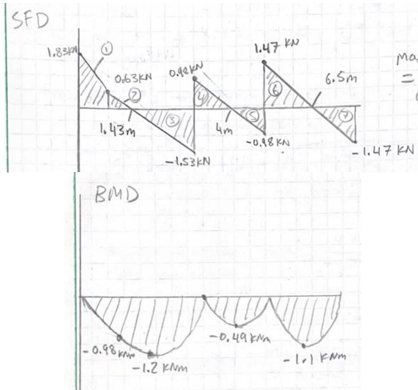
Figure 8: Factored Shear and Bending Diagrams for Front Girt (See Volume III on pg. 38)
