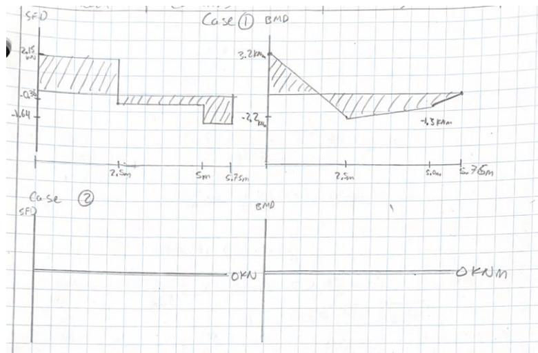
Figure 11: Factored Shear and Bending Diagram for 5.75m Long Column (See Volume III on pg. 53)
