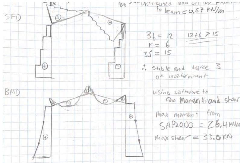
Figure 12: Shear and Bending Diagram for Middle Frame (See Volume III on pg. 57)
