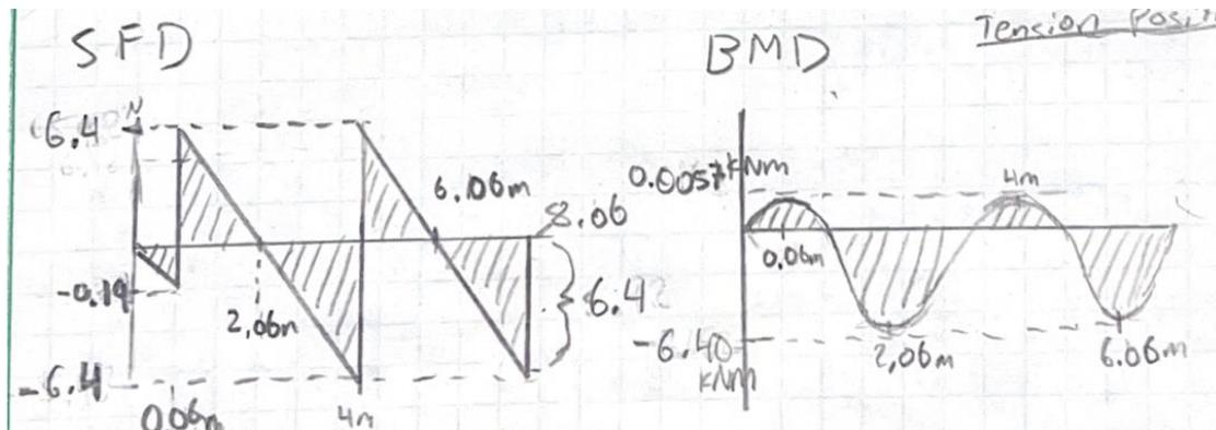
Figure 5: Factored Shear and Bending Diagrams for Purlin (See Volume III on pg. 20)
