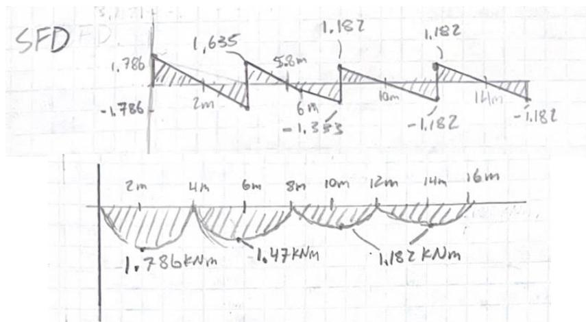
Figure 6: Unfactored Shear and Bending Diagrams for Side Girt (See Volume III on pg. 26, 27)
