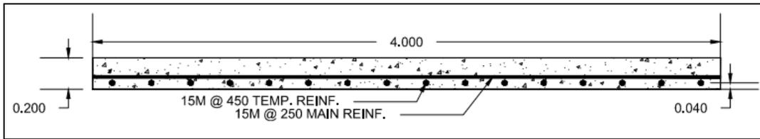
Figure 13: Concrete Pump Pad (See Volume II, 'Pump Pad Plan - Section A')
