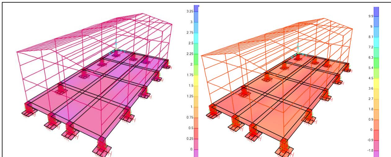
Figure 17: Deflection in the x and y Direction for 0.9D + 1.4W in SAP2000.
