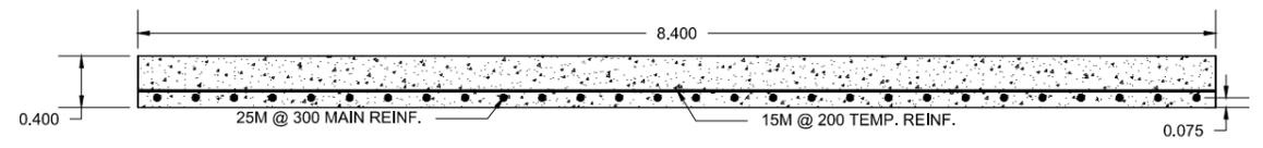
BASE SLAB PLAN - SECTION C1
