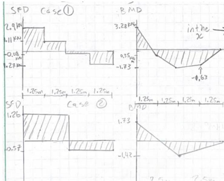
Figure 10: Factored Shear and Bending Diagrams for 5m Long Column (See Volume III on pg. 45)
