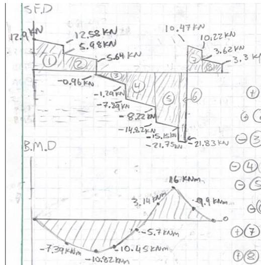
Figure 7: Factored Shear and Bending Diagrams for End Wall Rafter (See Volume III on pg. 32)
