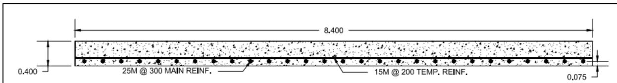
Figure 14: Concrete Base Slab (See Volume II, 'Base Slab Plan - Section C')
