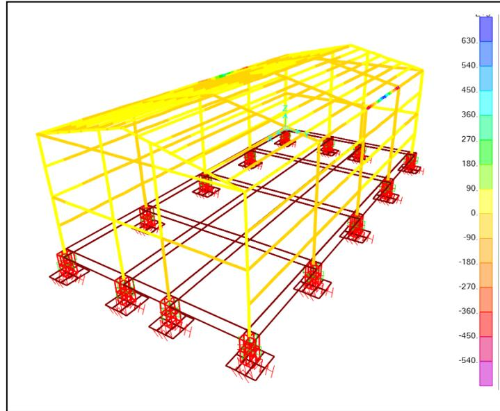
Figure 18: Stress in Steel Members for  $0.9D + 1.4W$  in SAP2000.
