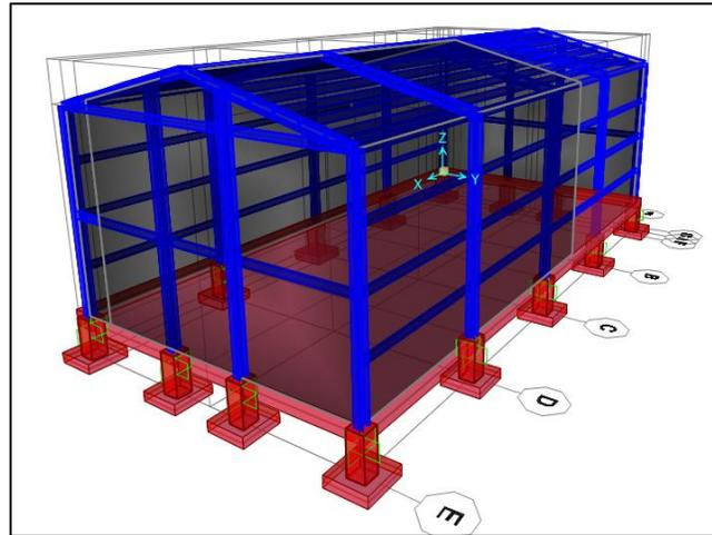
Figure 4: SAP2000 Model of Steel Structure (B. Mendoza)
