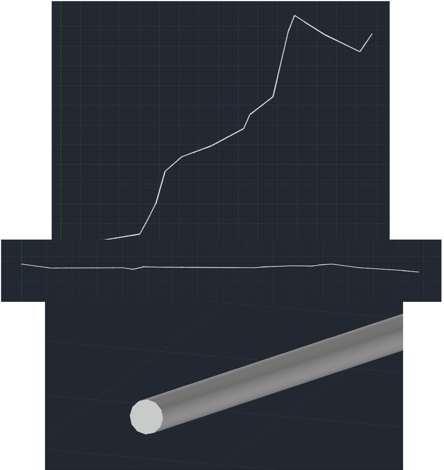
*Figure A1: Plan View, Profile View, and Closeup View of 200mm Pipe in AutoCAD.*
