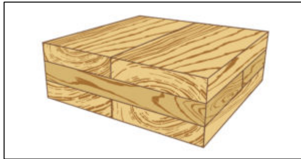
Figure 3: Visual of CLT panel layering (naturally:wood, n.d.)
