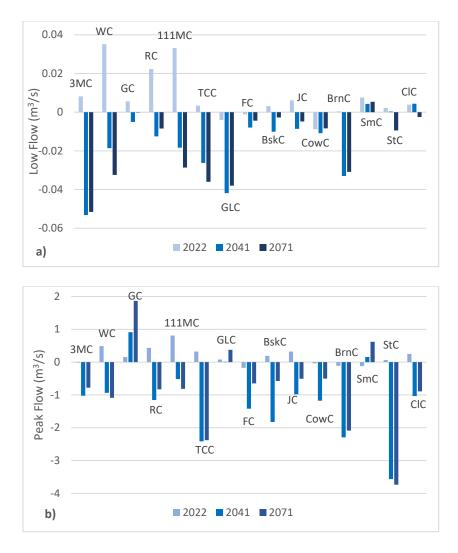
**Figure 14.** Bar charts of the 15 field sites showing (a) 2022 estimated low flows with climate data and 2041 and 2071 projected low flows by field site; (b) 2022 estimated peak flows with climate data and 2041 and 2071 projected peak flows by field site. Site codes shown in Section 4.7.
