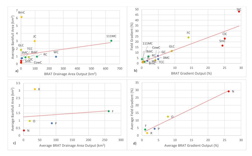
**Figure 3.** Scatter plots showing the correlation between (a) BRAT drainage area outputs and average bankfull area of assessed sites; (b) BRAT gradient outputs and field-measured gradient of assessed sites; (c) BRAT-estimated drainage area and bankfull area averaged by BRAT suitability; and (d) the average BRAT gradient outputs and field-measured gradients averaged by BRAT suitability.
