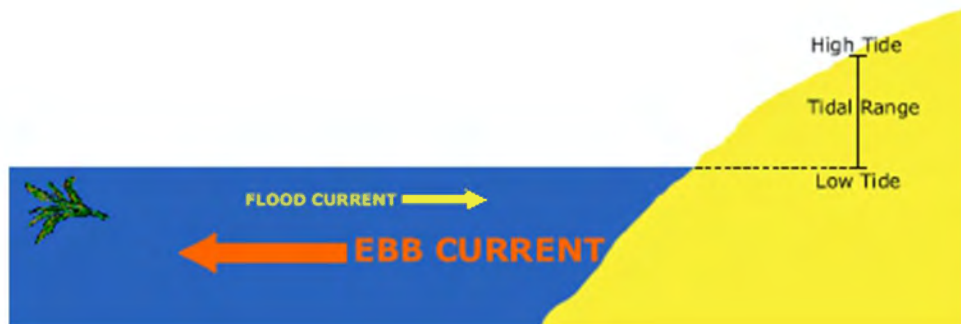
Figure 18. Correlation between spatial and temporal component of tides, as high tide results in water move toward the shore (flood current), low tides consequently cause water to move back from the shore (ebb current). (Animation by NOAA )
