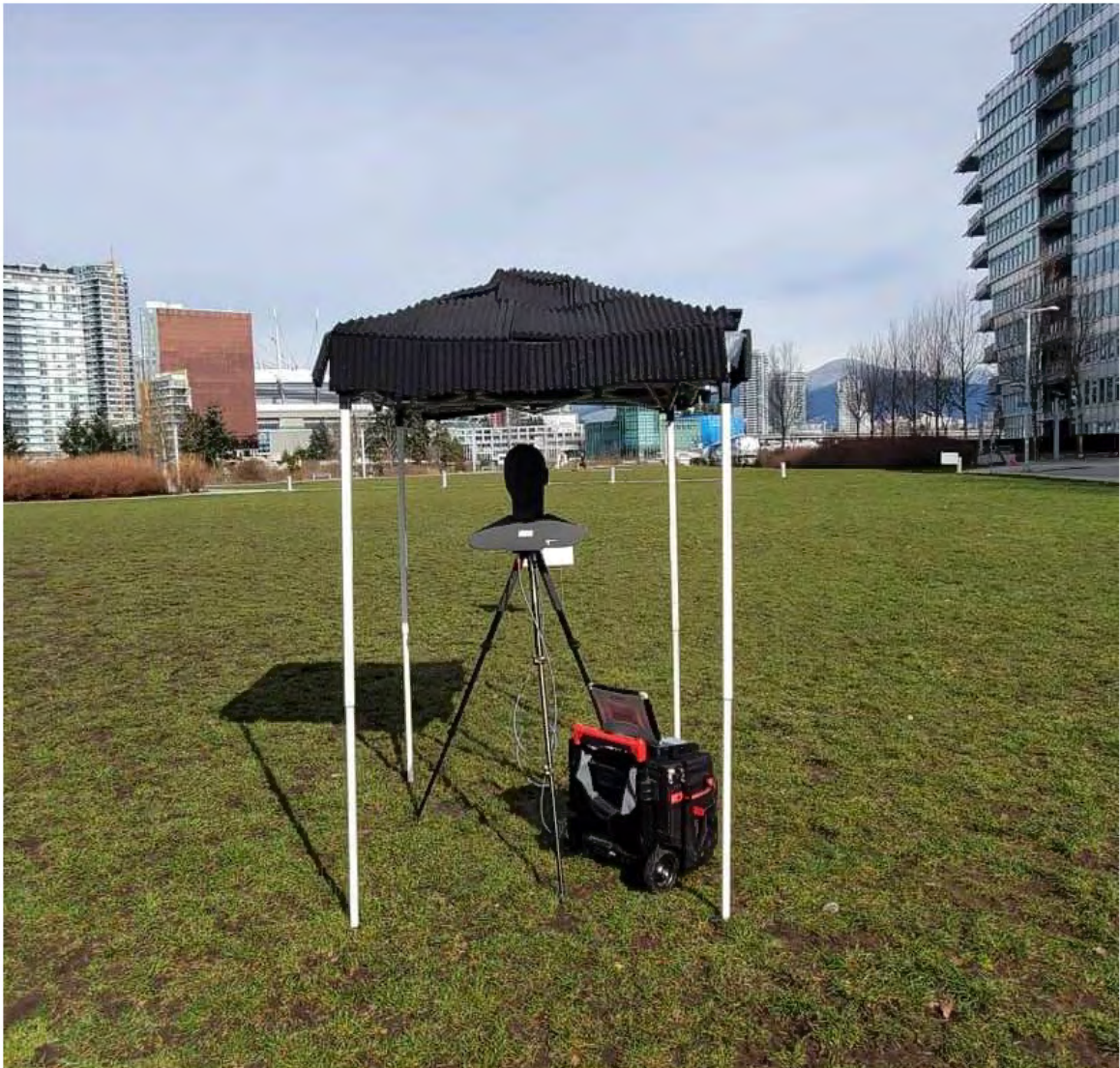
Figure 17. Equipment Setup in the Field (Soundbook placed on top of tools bag and connected to a binaural head mounted on tripod at height of 1.6m, covered with a sound absorption shelter)
