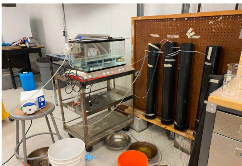
Figure 2.3: BCIT Civil Engineering lab filtration experiment set up.
