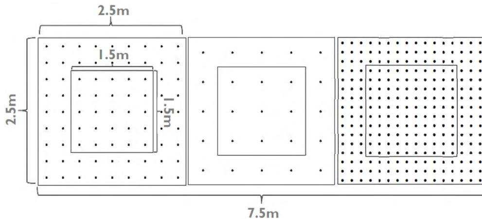
**Figure 3.1:** Diagram of block layout in density trials. Dots represent planted stakes in 30 cm, 50 cm, and 15 cm spacings (Adapted from Marcoux et al. 2017).
