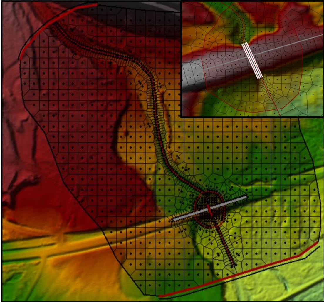
*Figure 8: 2D only model of Creek Y and Zoomed in 2D Model of Culvert X (top right)*
