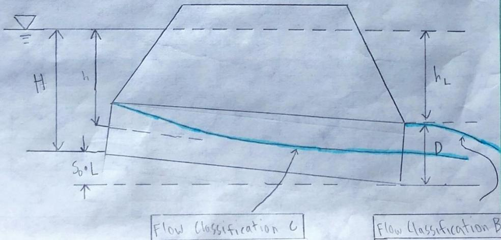
Assuming Full pipe flow or flow classification B), the energy balance can be expressed as:
