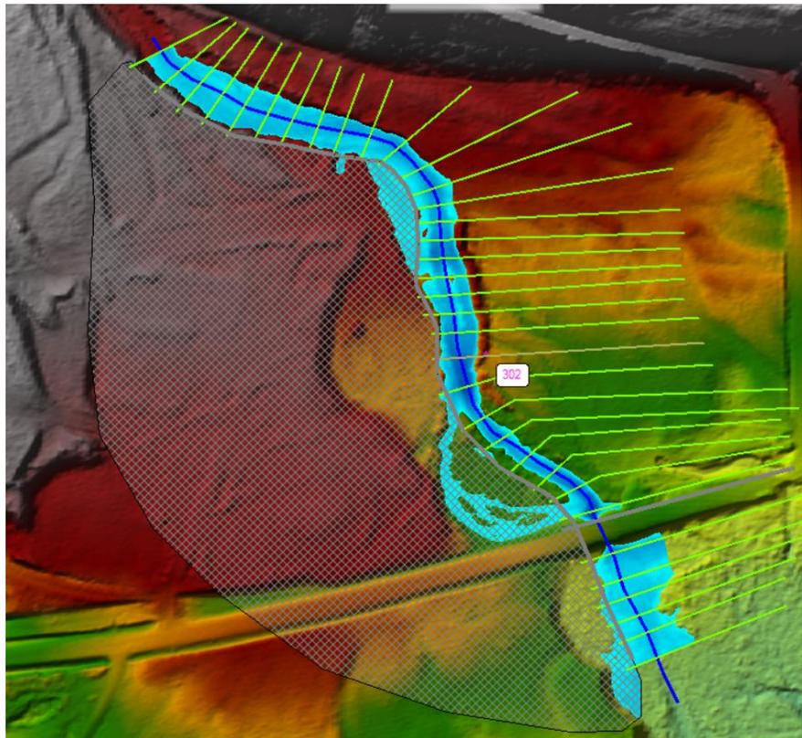
**Figure 11:** Maximum flood depth in Creek Y with newly designed culverts
