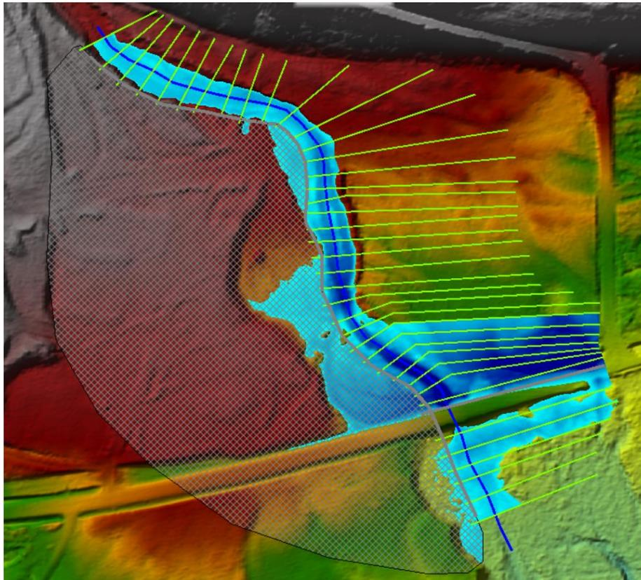
*Figure 10: Maximum flood depth in Creek Y with Original Flooding Culvert X*
