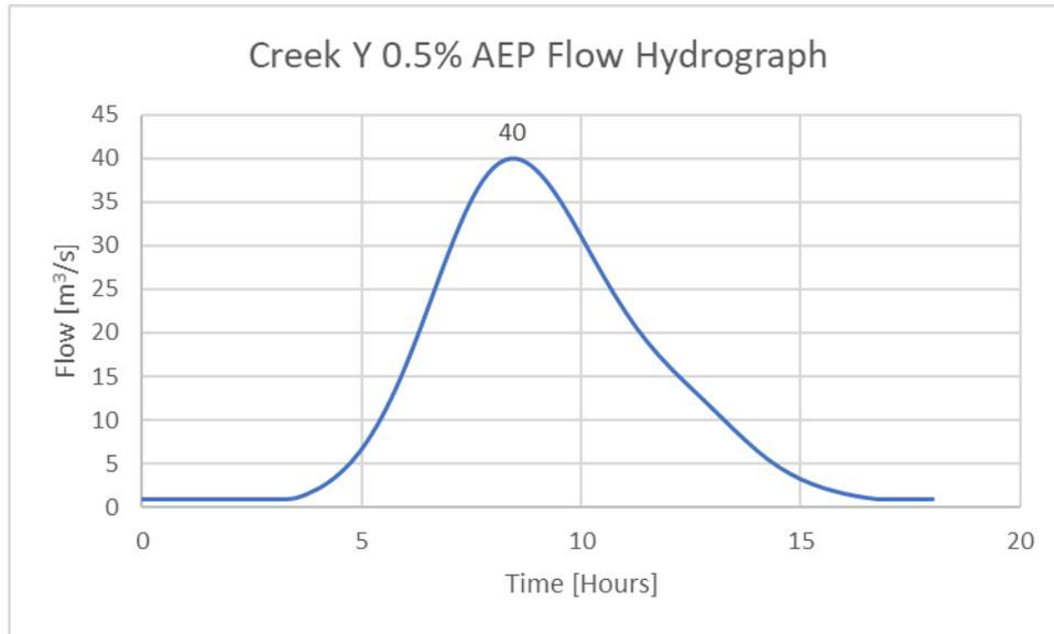
**Figure 3:** *0.5% AEP Flow Hydrograph for Creek Y*
