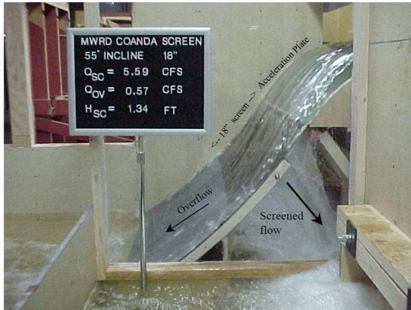
Figure 22 Experimental test of Coanda screens (Wahl, 2003)
