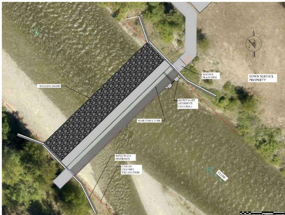
Figure 40 Overhead view of the weir structure
