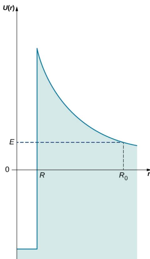
**Figure 7.18** The potential energy barrier for an  $\alpha$ -particle bound in the nucleus: To escape from the nucleus, an  $\alpha$ -particle with energy  $E$  must tunnel across the barrier from distance  $R$  to distance  $R_0$  away from the center.
