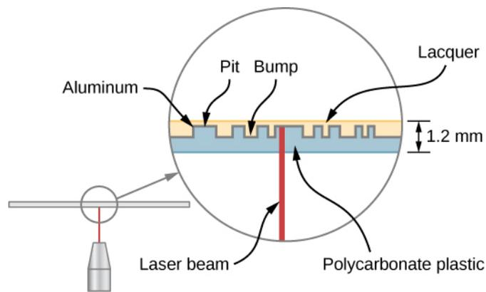
**Figure 8.30** A compact disc is a plastic disc that uses bumps near its surface to encode digital information. The surface of the disc contains multiple layers, including a layer of aluminum and one of polycarbonate plastic.
