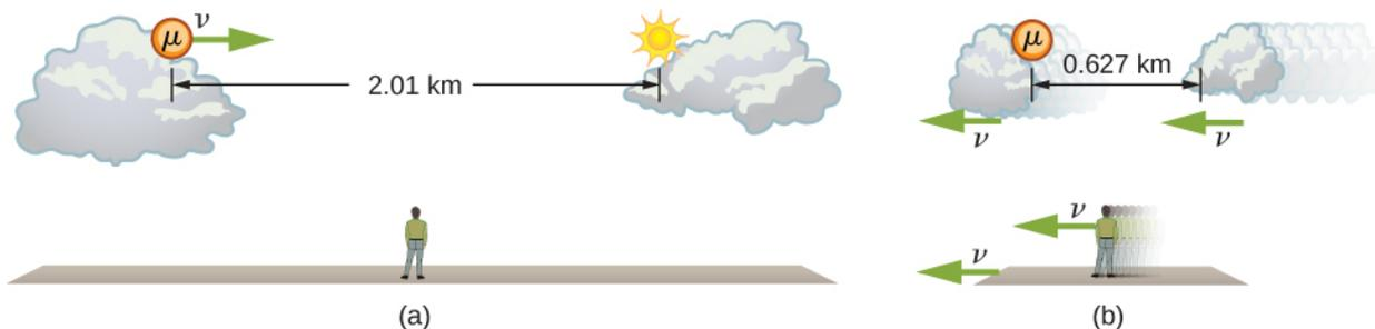
**Figure 5.9** (a) The earthbound observer sees the muon travel 2.01 km. (b) The same path has length 0.627 km seen from the muon's frame of reference. The Earth, air, and clouds are moving relative to the muon in its frame, and have smaller lengths along the direction of travel.
