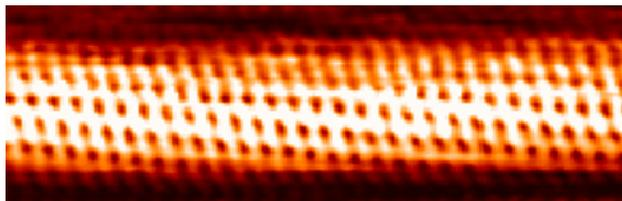
**Figure 7.22** An STM image of a carbon nanotube: Atomic-scale resolution allows us to see individual atoms on the surface. STM images are in gray scale, and coloring is added to bring up details to the human eye.
