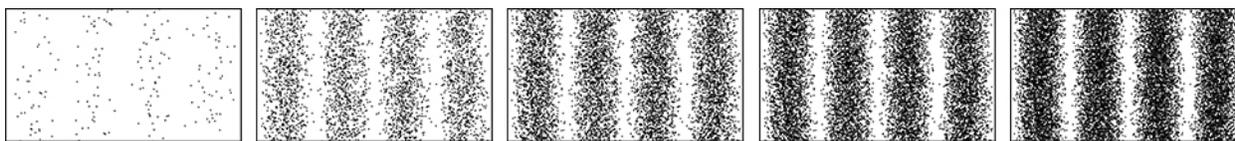
**Figure 6.24** Computer-simulated interference fringes seen in the Young double-slit experiment with electrons. One pattern is gradually formed on the screen, regardless of whether the electrons come through the slits as a beam or individually one-by-one.
