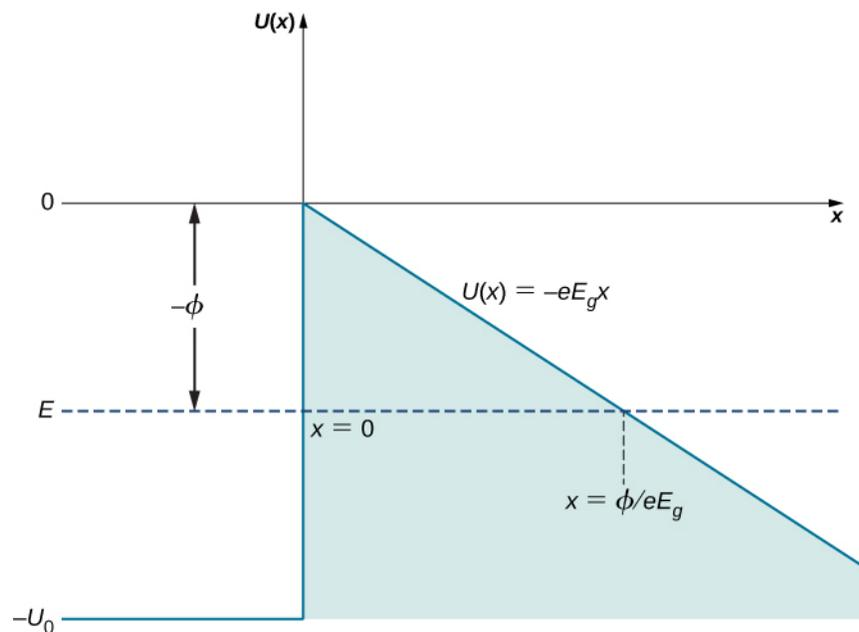
**Figure 7.20** The potential energy barrier at the surface of a metallic conductor in the presence of an external uniform electric field  $E_g$  normal to the surface: It becomes a step-function barrier when the external field is removed. The work function of the metal is indicated by  $\phi$ .
