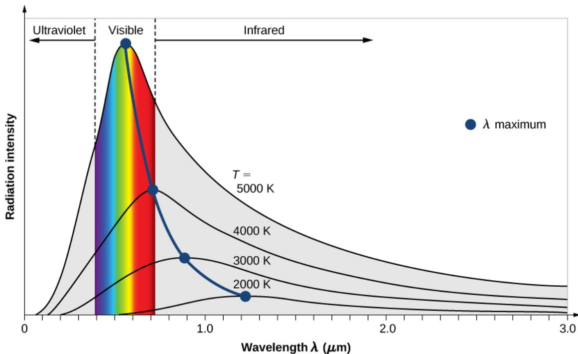
**Figure 6.3** The intensity of blackbody radiation versus the wavelength of the emitted radiation. Each curve corresponds to a different blackbody temperature, starting with a low temperature (the lowest curve) to a high temperature (the highest curve).
