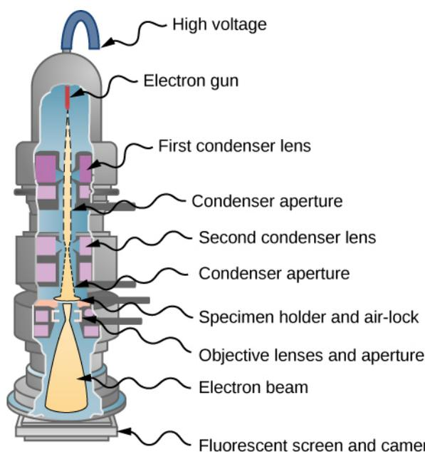
**Figure 6.26** TEM: An electron beam produced by an electron gun is collimated by condenser lenses and passes through a specimen. The transmitted electrons are projected on a screen and the image is sent to a camera. (credit: modification of work by Dr. Graham Beards)
