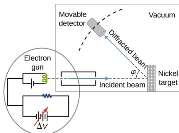
**Figure 6.19** Schematics of the experimental setup of the Davisson–Germer diffraction experiment. A well-collimated beam of electrons is scattered off the nickel target. The kinetic energy of electrons in the incident beam is selected by adjusting a variable potential,  $\Delta V$ , in the electron gun. Intensity of the scattered electron beam is measured for a range of scattering angles  $\varphi$ , whereas the distance between the detector and the target does not change.
