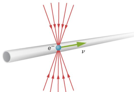
**Figure 5.12** The electric field lines of a high-velocity charged particle are compressed along the direction of motion by length contraction, producing an observably different signal as the particle goes through a coil.
