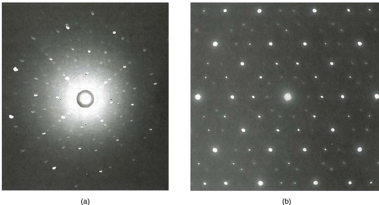
**Figure 6.22** Diffraction patterns obtained in scattering on a crystalline solid: (a) with X-rays, and (b) with electrons. The observed pattern reflects the symmetry of the crystalline structure of the sample.
