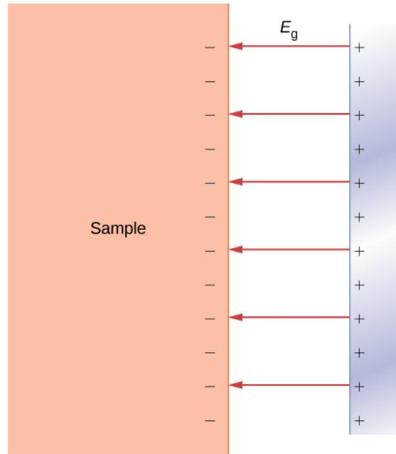
**Figure 7.19** A normal-direction external electric field at the surface of a conductor: In a strong field, the electrons on a conducting surface may get detached from it and accelerate against the external electric field away from the surface.
