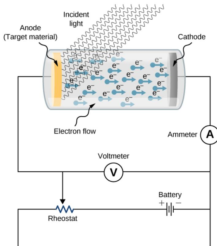
**Figure 6.8** An experimental setup to study the photoelectric effect. The anode and cathode are enclosed in an evacuated glass tube. The voltmeter measures the electric potential difference between the electrodes, and the ammeter measures the photocurrent. The incident radiation is monochromatic.
