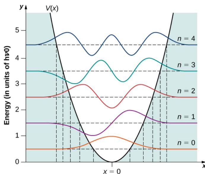
**Figure 7.14** The first five wave functions of the quantum harmonic oscillator. The classical limits of the oscillator's motion are indicated by vertical lines, corresponding to the classical turning points at  $x = \pm A$  of a classical particle with the same energy as the energy of a quantum oscillator in the state indicated in the figure.
