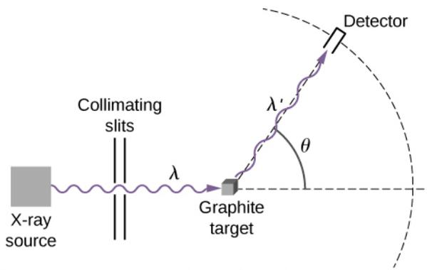
**Figure 6.11** Experimental setup for studying Compton scattering.
