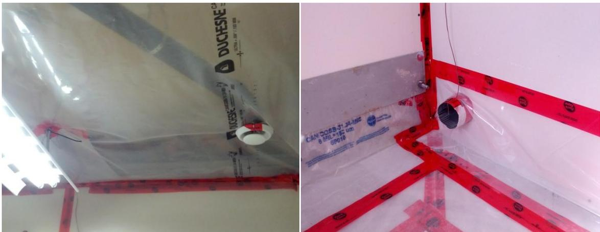
Figure 24. Locations of the diffuser on the ceiling (bottom left) and return vent on the partition wall (bottom right) and indicated on floor plan (top)
