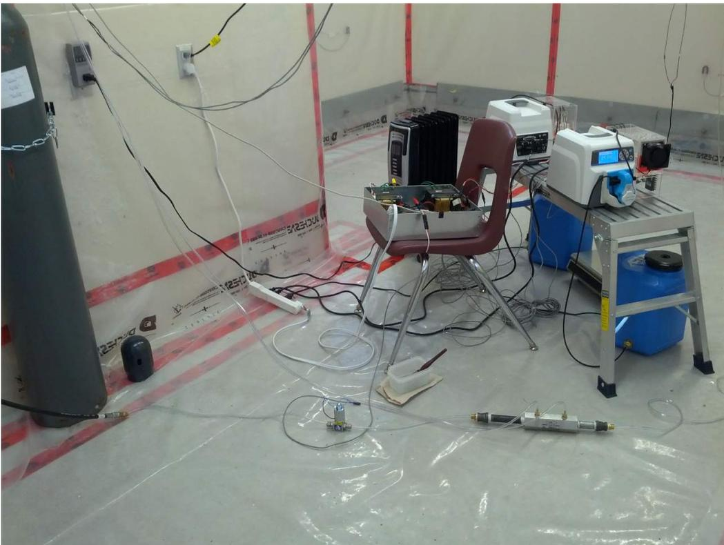
Components of the Occupant Simulator Unit in the Control (North) Building
