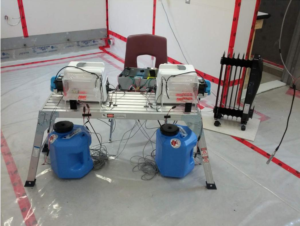
Components of the Occupant Simulator Unit in the Control (South) Building
