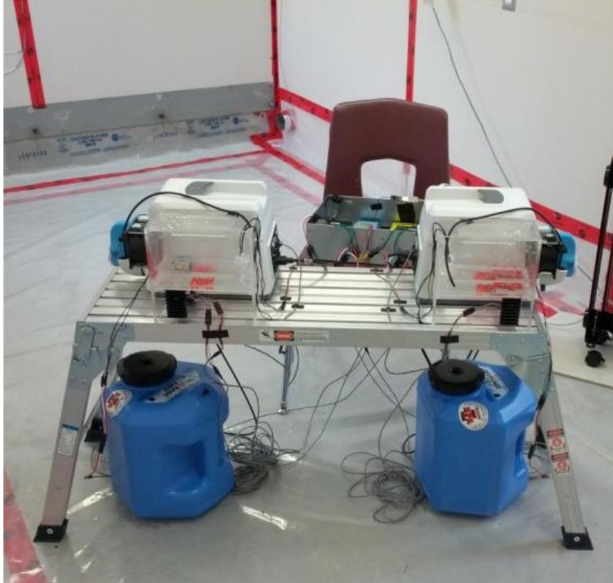
**Figure 26. Occupant simulator equipped with control box, humidifiers, water reservoirs, pumps, CO<sub>2</sub> release valve (not shown), and heat generating bulb (not shown)**
