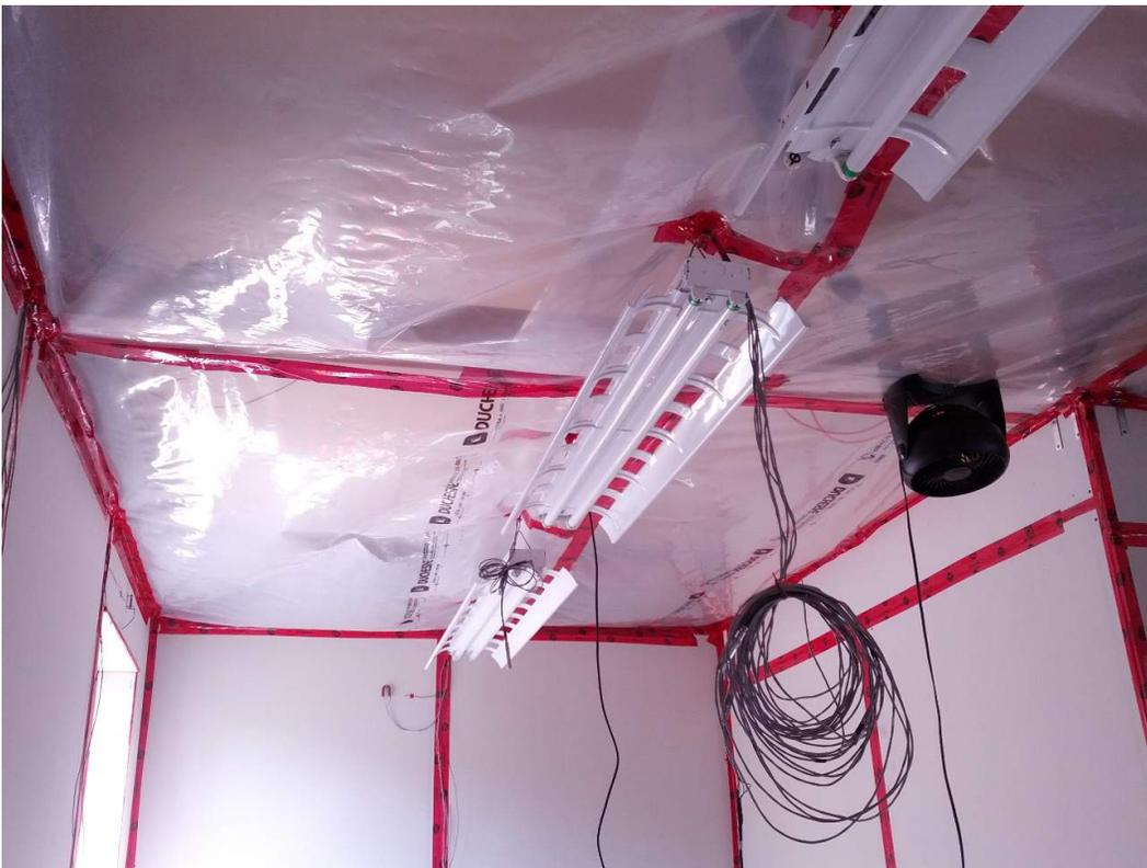
RHT Sensors Suspended From Ceiling used for Measurement of Interior Conditions
