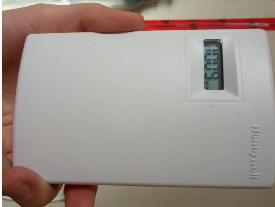
**Figure 39. CO<sub>2</sub> Sensor can measure and record CO<sub>2</sub> concentration**
