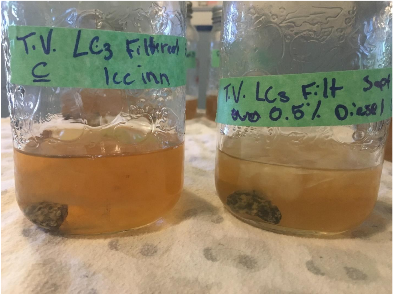
Figure 20. Comparison of mycelial growth in liquid media, no diesel on the left and diesel of on the right.
