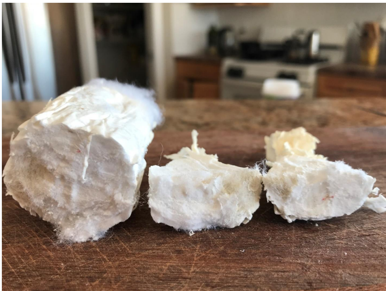
Figure H-3. Cross section close-up of T. versicolor having colonized a polyfill air filter.
