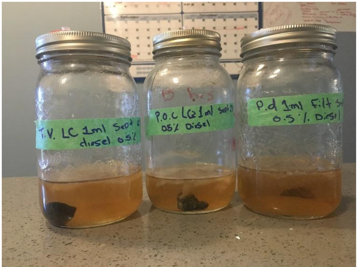
Figure 19. Mycelium growing mainly on the top surface of liquid culture during the priming process with 0.5% diesel, after 14 days.
