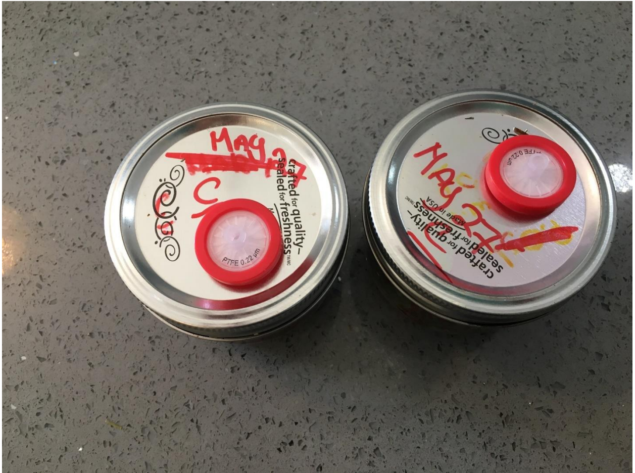
Figure 14. Mason jars with lids with fitted with 0.22-micron air filters.
