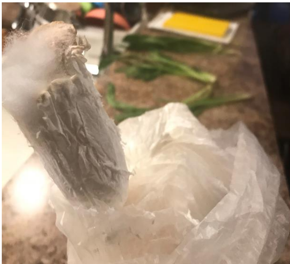
Figure H-2. Close up of the how T. versicolor colonization of the polyfill air-filter, possibly consuming the material.
