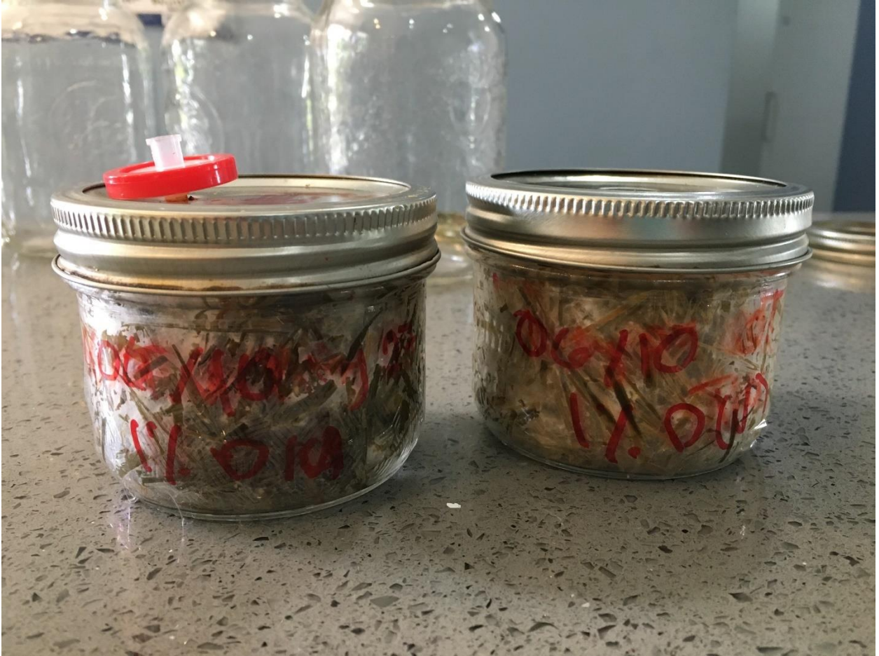
Figure 15. Colonized hay ( T. versicolor ) during the priming process at 1 percent diesel, June 10 th , 2019.
