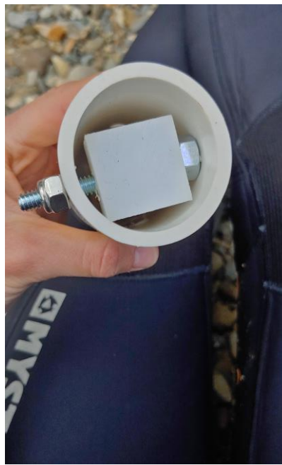
Photo 4 - White insert with logger bolted into top holes of PVC pipe.
