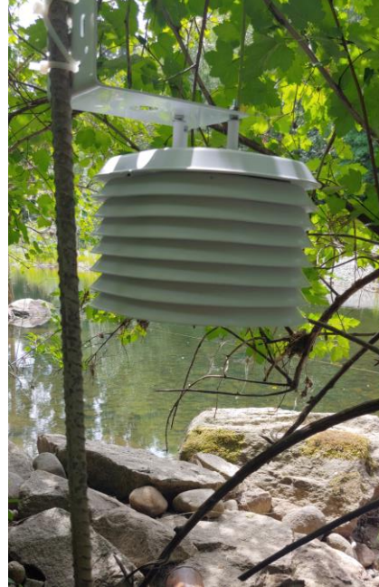
Photo 6 – A2-2019 installed within solar radiation shield along covered bank, looking southwest.
