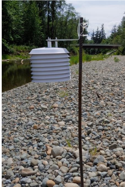
Photo 5 – A1-2019 installed within solar radiation shield on exposed gravel bar, looking south.
