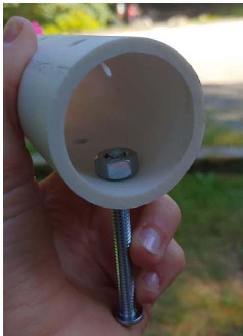
Photo 1 - PVC pipe with bolt and spacer prior to logger insertion.
