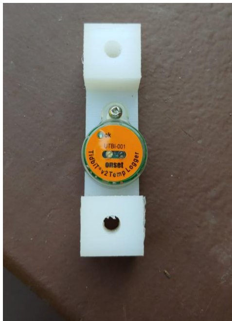
Photo 2 - Logger attached to white insert that was installed inside PVC pipe.
