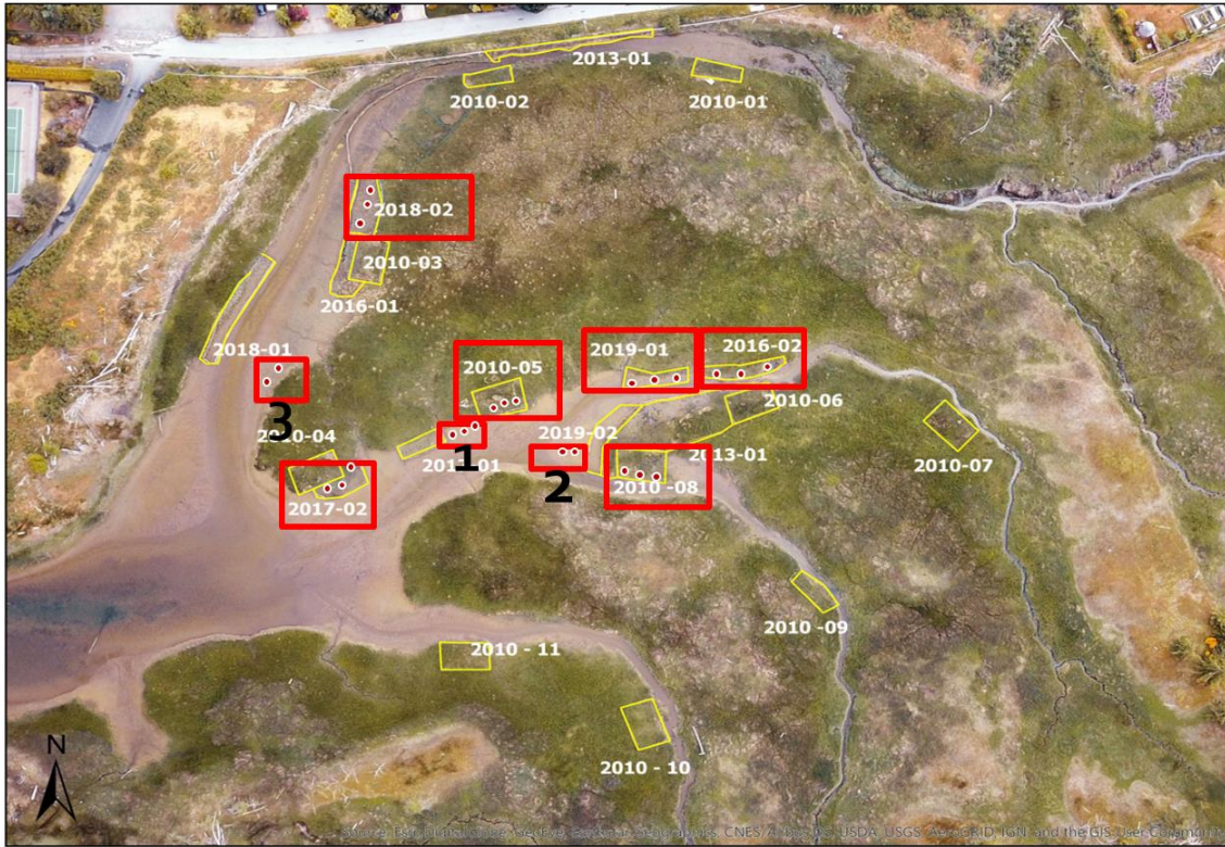
Figure 2.3 Sediment traps (red dots) were deployed at each sampling location (outlined in red boxes) to compare rates of deposition inside exclosures installed in different years and along three denuded mud flat locations in the Little Qualicum River Estuary, Vancouver Island, BC in the summer of 2019.
